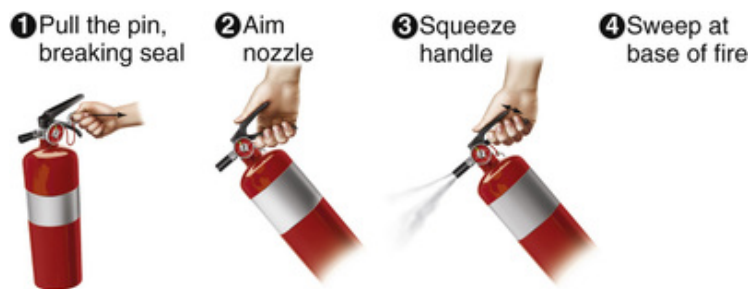
FIGURE 25.7 When using a fire extinguisher, remembering the PASS acronym (i.e., pull, aim, squeeze, and sweep) ensures proper technique.
