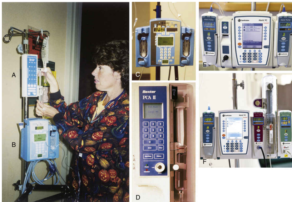
FIG. 11.12 Electronic Infusion Devices. (A) Syringe pump. (B) Single-channel infusion pump. (C) Dual-channel infusion pump. (D) Patient-controlled analgesia (PCA) pump. (E) Alaris system. (F) Alaris system with PCA module.
