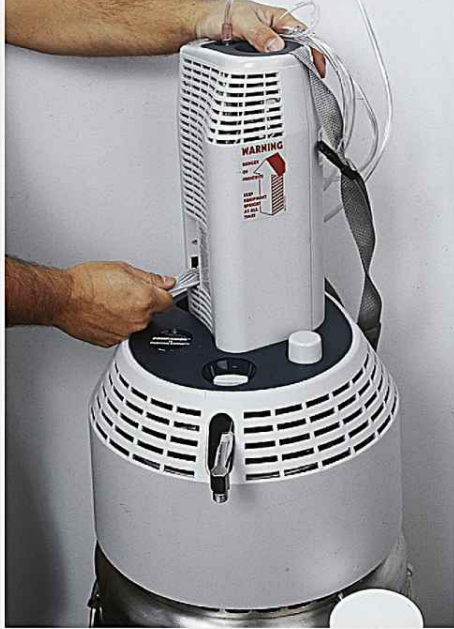
Step 3c(3)(d) Fill valve on ambulatory tank is opened while applying firm pressure to top of ambulatory unit.
