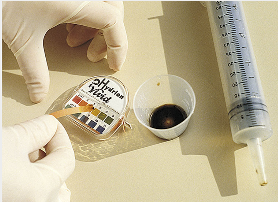
STEP 11D Compare color on test strip with color on pH chart.
