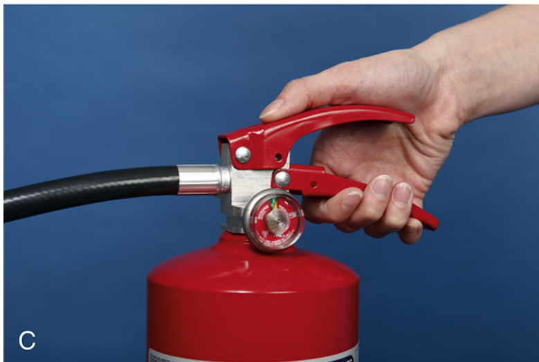
FIG. 27.8 Correct use of a fire extinguisher. A , Pull pin. B , Aim at base of fire. C , Squeeze handles and Sweep from side to side to coat area evenly.
