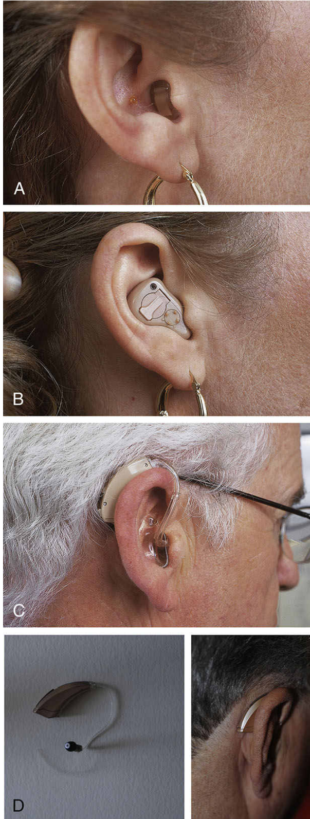
FIG. 40.6 Common types of hearing aids. A , Completely-in-canal (CIC) hearing aid. B , In-the-ear (ITE) hearing aid. C , Behind-the-ear (BTE) hearing aid. D , Digital hearing aid.
