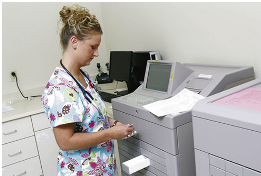
FIG. 31.6 Automated medication dispensing system (AMDS).
