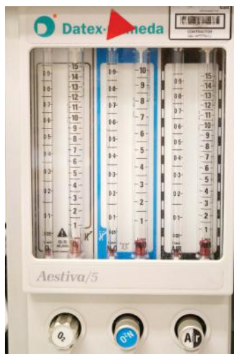
Fig. 6.3.1: A bank of flowmeters mounted on the front of the anaesthetic machine. Small meters read from 0.05 \text{ l.min}^{-1} to 1 \text{ l.min}^{-1} , while the large meters read from 1 \text{ l.min}^{-1} to 15 \text{ l.min}^{-1} .
