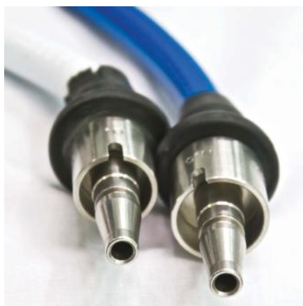
Fig. 1.6.2: Oxygen and nitrous oxide Schrader probes. The hoses are colour coded and the probes labelled with the gas name. The different diameter index collar physically prevents cross-connection.
