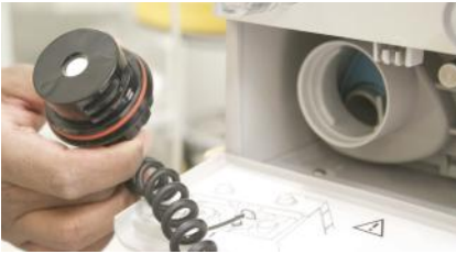
Fig. 6.4.1: The fuel cell removed from covering on anaesthetic machine.
