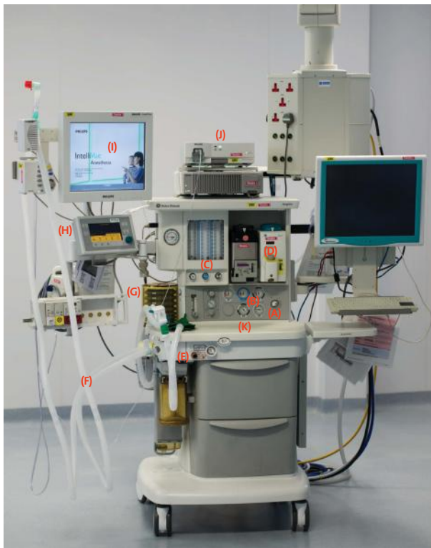
Fig. 5.2.1: A GE Datex Ohmeda Aespire machine. Components include (A) on/off switch, (B) pipeline and cylinder pressure gauges, (C) flowmeters, (D) vaporizers mounted on the back bar, (E) common gas outlet (not in use), (F) circle system, (G) bag in bottle ventilator, (H) ventilator controls, (I) monitor, (J) gas module (for monitoring anaesthetic gases), and (K) suction control.
