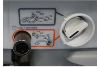
Fig. 5.2.10: A common gas outlet. The switch indicates the gas will exit the outlet rather than being diverted through the built-in circle system.
