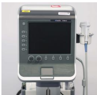
Fig. 11.2.1: The Sonosite S-Nerve ultrasound machine is specifically designed for anaesthetics and has settings for nerve blocks and vascular access.
