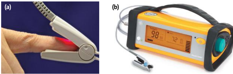
Fig. 6.10.1: (a) A pulse oximeter on a finger. (b) The TruSat pulse oximeter. Image reproduced with permission from GE Healthcare.
