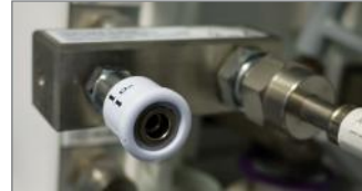
Fig. 5.2.11: A mini-Schrader valve attached to the oxygen supply on an anaesthetic machine. On some machines, the valve is built in.
