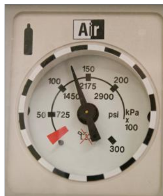
Fig. 6.2.2: A Bourdon gauge found on the front of the anaesthetic machine showing air cylinder pressure.
