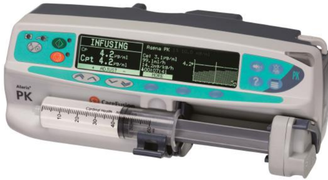
Fig. 5.12.1: The Alaris PK (pharmacokinetic) pump (Carefusion). A target plasma propofol concentration (Cpt) of 4.2 \mu\text{g}\cdot\text{ml}^{-1} has been set. The Cp is also 4.2 \mu\text{g}\cdot\text{ml}^{-1} , indicating that the pump has calculated that the plasma concentration has reached this target. This is graphically illustrated on the right of the screen which shows the set concentration (horizontal line) and calculated concentration (shaded area) over the last 5 minutes. The Ce (effect site concentration) is also displayed. At this point the Ce is only 3.1 \mu\text{g}\cdot\text{ml}^{-1} , indicating that a steady state at the effect site has yet to be reached. The decrement time is indicated at 7 minutes 41 seconds; this is the predicted time for the target concentration to fall to a set value, usually 1 \mu\text{g}\cdot\text{ml}^{-1} . It gives an indication of the time to wake up if the pump is switched off. Image courtesy of Carefusion.
