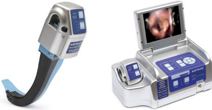
Fig. 2.9.1: An Airtraq laryngoscope with optional camera attachment. The image is wirelessly transmitted to the monitor. Image courtesy of Airtraq.
