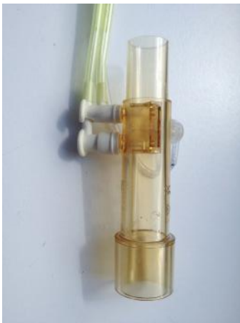
Fig. 6.15.2: Pitot tubes. This connects to a breathing system. The yellow tubing connects to the differential pressure transducer.
