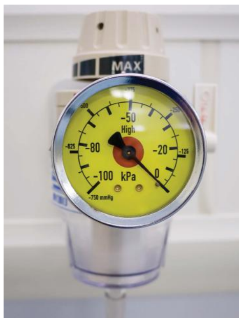
Fig. 1.7.1: A wall suction unit showing the variable pressure regulator and suction trap.
