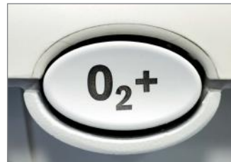
Fig. 5.2.6: A recessed oxygen flush button on the front of an anaesthetic machine.
