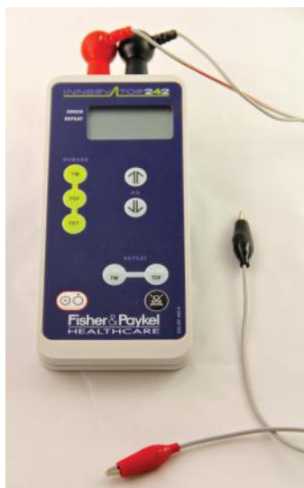
Fig. 8.1.2: A nerve stimulator used for monitoring neuromuscular blockade.
