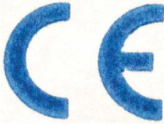
Fig. 12.7.1: The CE mark. A product bearing this symbol has been manufactured to standards that conform with European Union legislation.
