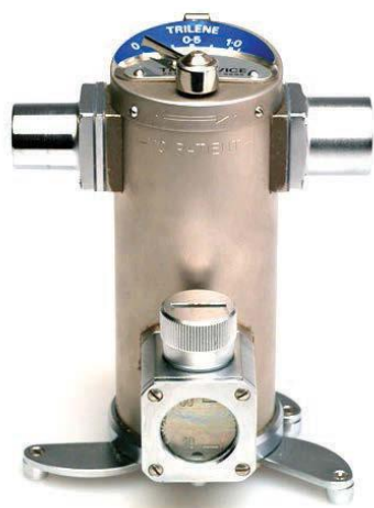
Fig. 5.9.1: The Oxford Miniature Vaporizer. Image courtesy of the Anaesthesia Museum, Sheffield Teaching Hospitals NHS Foundation Trust.
