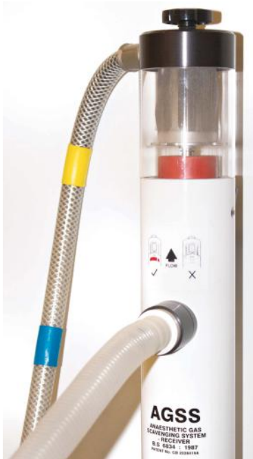
Fig. 1.8.2: An open receiving system (the opening is at the bottom of the device, not shown in the image). The 30 mm corrugated hose connects to the APL valve and the top hose connects to the active disposal system.
