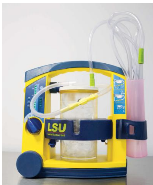
Fig. 1.7.2: The Laerdal suction unit (Laerdal Medical) is a battery operated portable suction unit.
