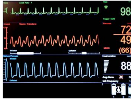
Fig. 9.19.2: An intra-aortic balloon pump monitor showing ECG (top trace, green), arterial pressure with diastolic augmentation (middle trace, red), and balloon inflation pressure (bottom trace, blue).
