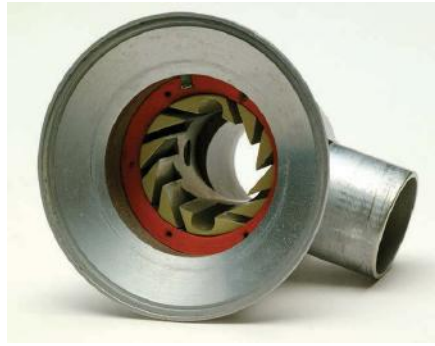
Fig. 6.16.2: A Wright respirometer with front removed so that workings can be seen. Image reproduced with permission from the Anaesthesia Museum, Sheffield Teaching Hospitals NHS Foundation Trust.
