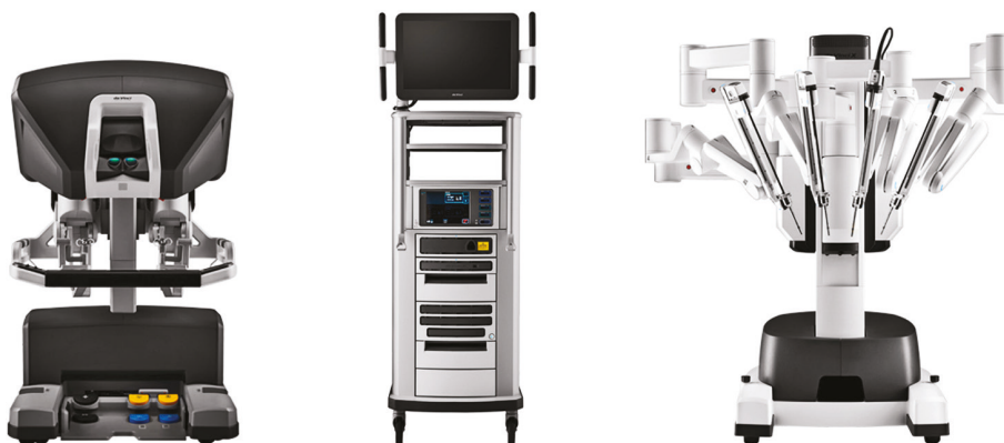
Figure 21.2 The Da Vinci Xi Robotic Surgical System (Intuitive Surgical, Mountain View, CA, US). From left to right: surgeon console, vision cart, patient cart.
