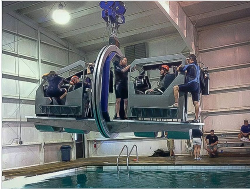
Figure 47.4 Dunker training for aviation skills – Apache Modular Egress Training Simulator (Apache METS®) by Survival Systems, Inc.
