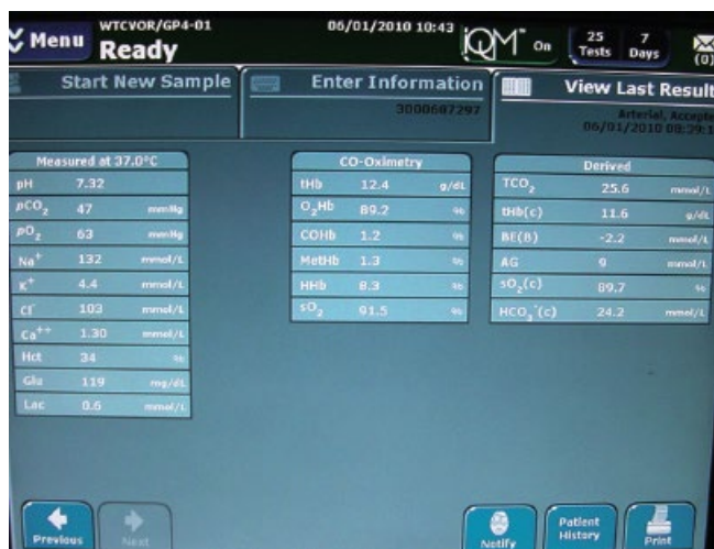
Figure 19.17 Point-of-care monitor for blood gases, electrolytes, hematocrit, ionized calcium, glucose, lactate, co-oximetry. 0.5 mL heparinized blood sample, 80 s measurement time, temperature correction.
