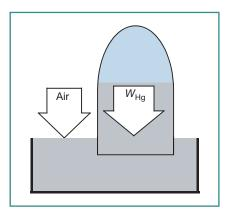
Figure 3.2 A Barometer
