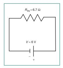
Figure 10.9 Parallel Resistors (Reduced Circuit)
