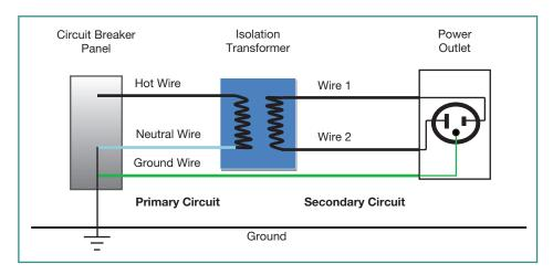
Figure 10.24 An Isolated Ungrounded Electrical Circuit
