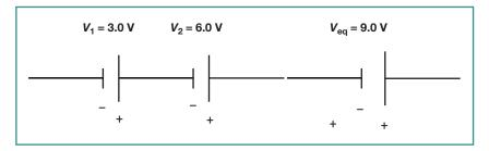
Figure 10.6 Batteries Connected in Series
