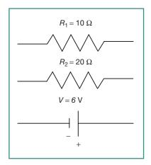
Figure 10.8 Parallel Resistors
