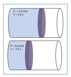
Figure 4.1 Expanding Gases and Work
