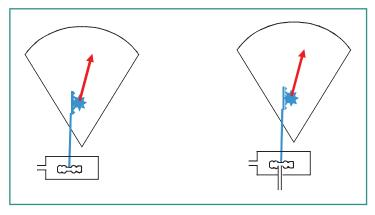
Figure 3.4 Aneroid Barometers
