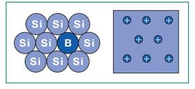
Figure 10.13 p-Type Semiconductor
