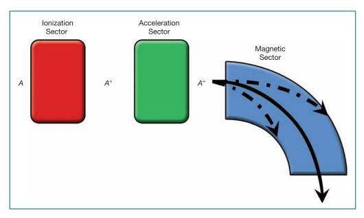
Figure 2.2 Schematic Diagram of Mass Spectrometer
