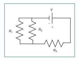
Figure 10.10 Parallel and Series Circuit
