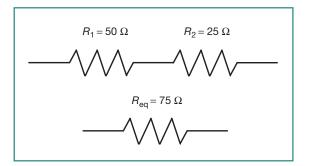
Figure 10.7 Resistors Connected in Series
