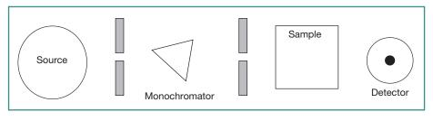
Figure 10.18 Schematic of a Spectrometer
