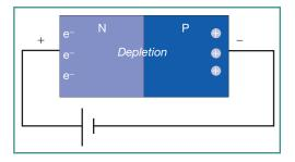
Figure 10.16 Reverse-Biased Diode
