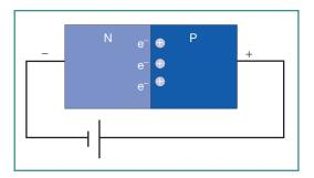
Figure 10.15 Forward-Biased Diode
