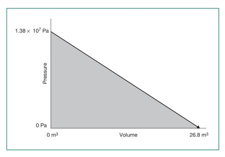
Figure 4.6 Work Done by the Rupture of a Gas Cylinder
