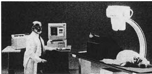
Fig. 13. The Lunar Expert, a fan-array DXA device. Photo courtesy of Lunar Corp.
