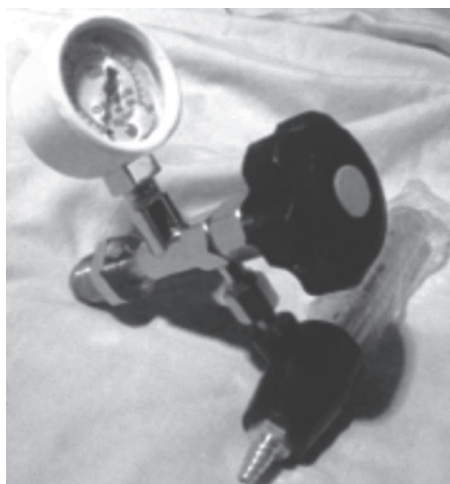
Fig. 1.10A: Bourdon pressure gauge
