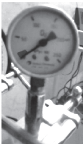
Fig. 1.9: Bourdon pressure gauge
