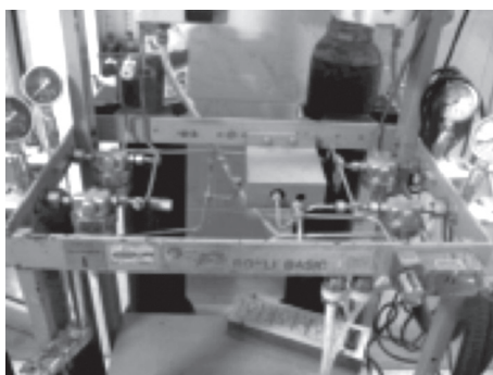
Fig. 1.18: Oxygen failure alarm
