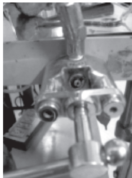
Fig. 1.8B: Pin index system (Yoke assemble)
