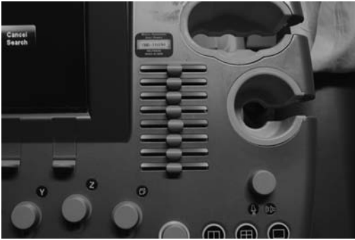
Figure 7.2. TGC Control. These 'sliders' are used to give a boost to returning echoes from different depths.
