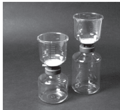
FIGURE 24-1 Sterile disposable vacuum filters (0.2- \mu\text{m} filter; 500-mL volume).
