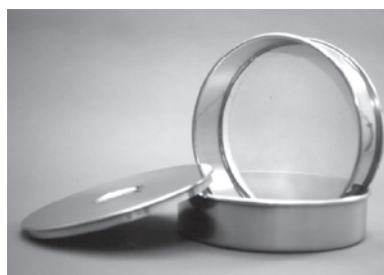
FIGURE 11-1 Brass sieve (No. 80 mesh).
