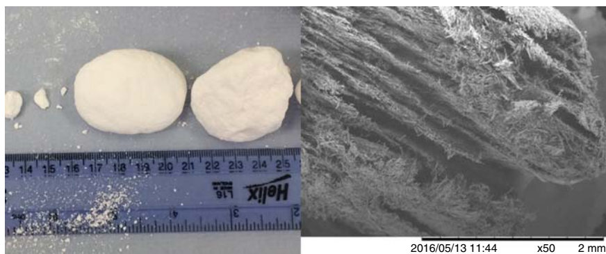
Figure 5.12 Lumps formed as a result of compression on the centrifuge.
