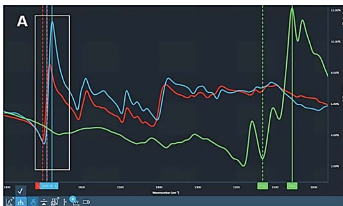
Figure 4.4.9 Diffuse reflectance infrared spectra of cellulose (green line), carbamazepine polymorph I (red) and III (blue). Source: Agilent Technologies, Inc. [13].
