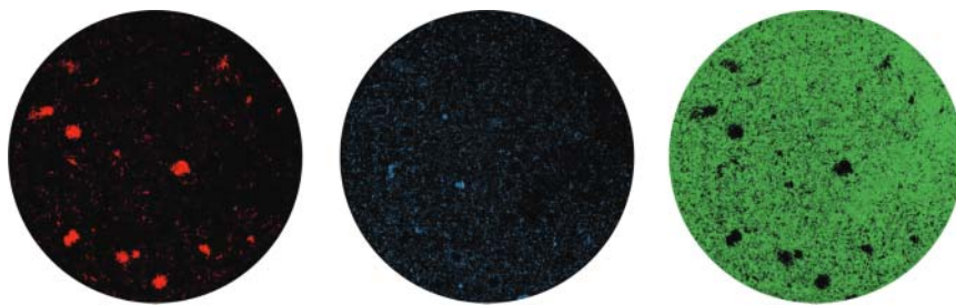
Figure 4.4.11 From left to right: Individual chemical maps of carbamazepine polymorph I, polymorph III and cellulose. Source: Agilent Technologies, Inc. [13].
