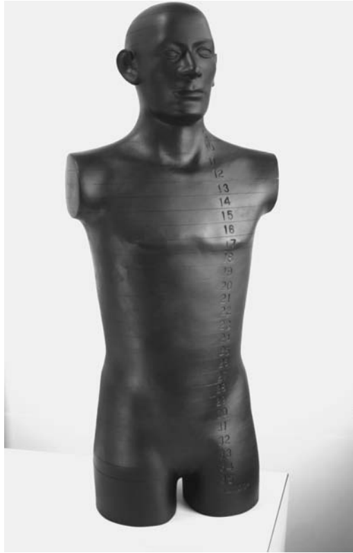
FIGURE 4.4 The male RANDO anthropomorphic phantom used in the brake radiation measurements. Each section of the phantom is 2.5 cm thick with positions for cylindrical TLD insertion being located in each slice. (Courtesy of Phantom Labs Inc. With permission.)
