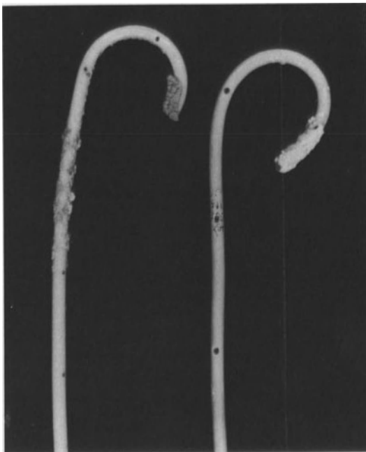
Fig. 3.14. Encrustation of the proximal ends of two stents removed from chronic stone-formers. Much of the external encrustation broke off during handling. The portions within the renal pelvis and bladder were heavily encrusted while the middle segment had been wiped clean by ureteral peristalsis. This phenomenon has been noted on numerous occasions and stents have been designed with external grooves to permit improved drainage in the face of encrustation. (From Finney R (1982) Double-J and diversion stents. Urol Clin North Am 9:89–94, with permission.)
