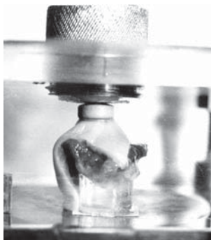
Figure 12.13 A device to measure the force of detachment of tablets or capsules from porcine oesophageal tissue, used to determine the values given in Fig. 12.14.
