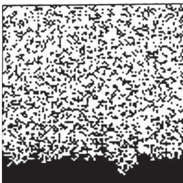
Figure 8.36 Theoretical representation of a polymer matrix: changes during erosion (dark pixels = nondegraded areas, white pixels = degraded areas), where \lambda_0 (a rate constant) = 2.7 \times 10^{-7} \text{ s}^{-1} for a sample containing 50% polyanhydride CPP.
