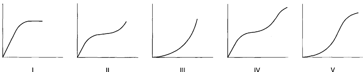
Fig. 5.13 Classification of isotherms for the adsorption of vapours by solids. Ordinates x/m , abscissae p/p_o .
