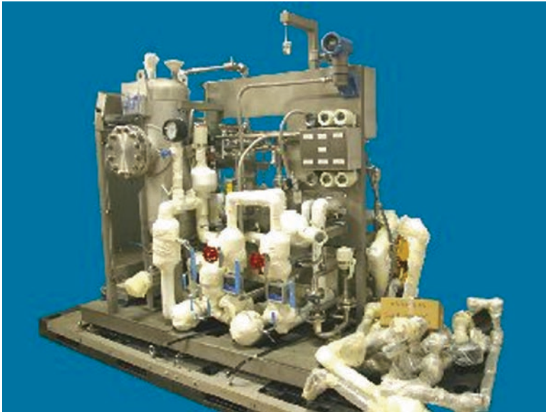
Fig. 8.6 Submicron media mill, high pressure supercritical fluid (SCF) processing. MAWP 6,000 psi @ 300 F. Reduces active pharmaceutical ingredients (API) to submicron size. Designed for class 10,000 area for flexibility and adherence to cGMP. Internal product wetted surfaces have 25–30 micro inch. RA finish. External surfaces have 50 micro inch Ra finish. Entire process is designed to accommodate four (4) skids on wheels. This can be used for Nano-suspensions with dispersed particle size in nanometer range
