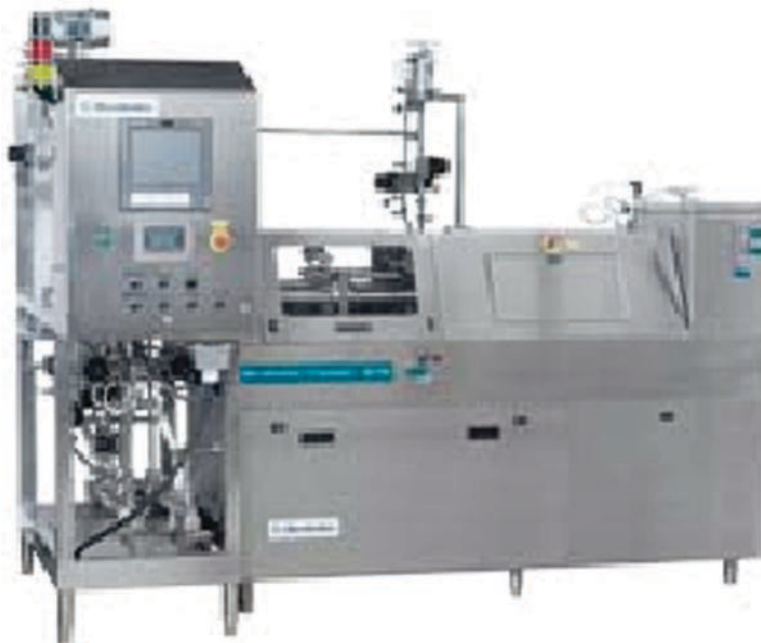
Fig. 5.11 Industrial scale Microfluidizer processor with steam sterilization (with permission from Microfluidics, Newton, MA)
