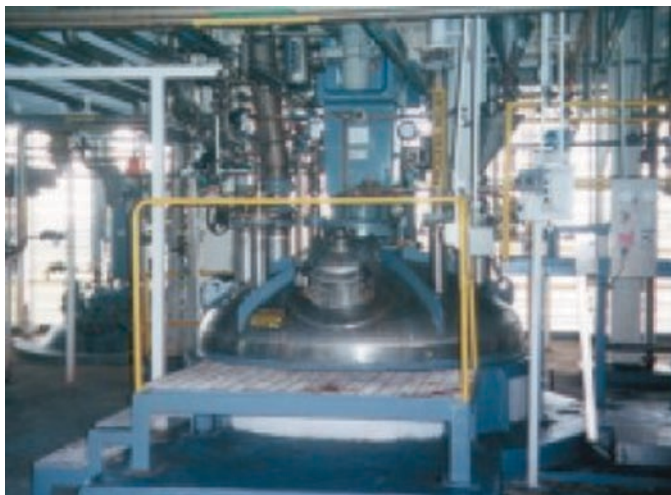
Fig. 8.3 Typical jacketed vessel for suspension manufacture with all the piping and processing alternative, it can be used for continuous or batch processing of suspensions
