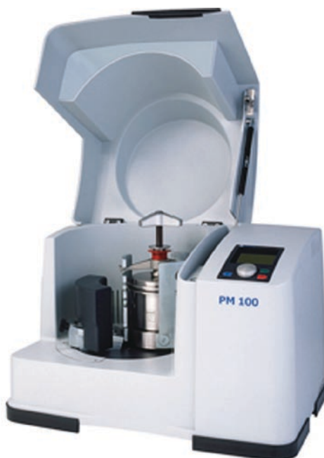
Fig. 5.7 Ball mill (wet and dry milling)
