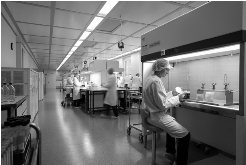
Figure 5.2 Example of laminar flow hoods within a microbiological laboratory. Source: Courtesy of BAV Institut GmbH Offenburg, Germany.
