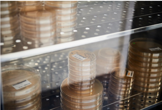
Figure 5.5 Solidified pour-plated agar plates in the incubator. Source: Courtesy of BAV Institut GmbH Offenburg, Germany.
