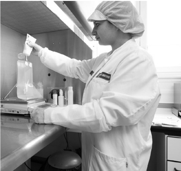
Figure 5.3 Weighing of a cream in a sample container placed on a precision balance. Source: Courtesy of BAV Institut GmbH Offenburg, Germany.
