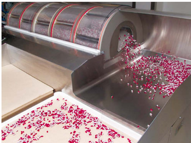
Figure 3.7 Photograph of soft capsule tumble drying. Image courtesy of Catalent.
