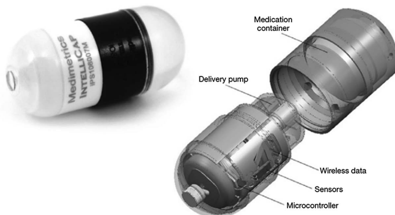
Figure 8.23 Picture and schematic illustration of the IntelliCap® system (dispensing type). 1 Published with permission from Medimetrics Personalized Drug Delivery B. V.
