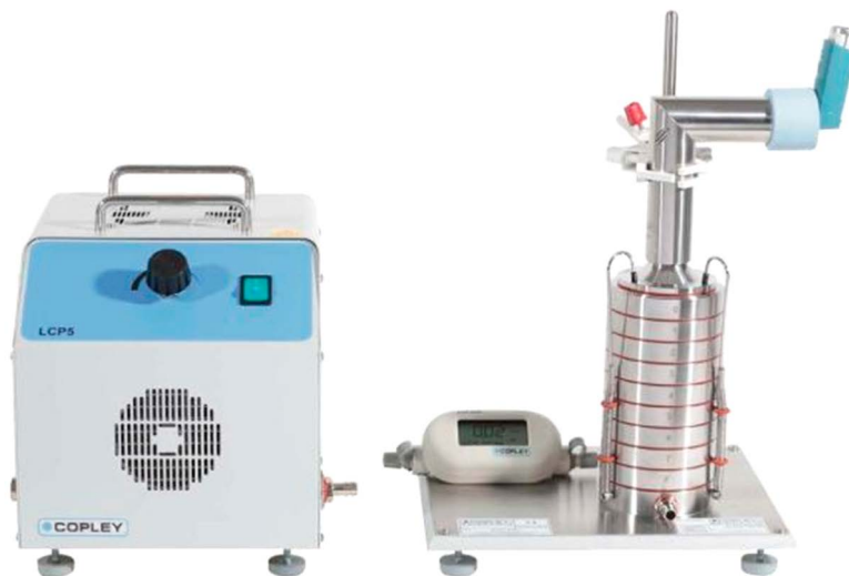
Figure 9.10 The Andersen Cascade Impactor (left). The basic configuration of the British Pharmacopoeia Apparatus D with modifications for use with dry powder inhalers (right). The dry powder inhaler is attached to the impactor using a standard throat and attachment port. The impactor draws air through the device by means of a vacuum pump connected to a rate-controlled air flow. With the permission of Copley Scientific.
