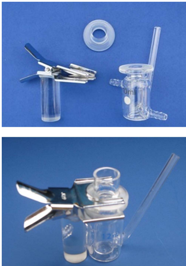
Figure 9.1 The Franz cell. The top image shows the component parts: the receptor half-cell and sampling port (lower right); the flange clip and support (lower left) and the donor half-cell. The lower image shows the assembled cell. The membrane is compressed between the donor and receptor cell flanges and clipped. Reproduced with the permission of Soham Scientific.
