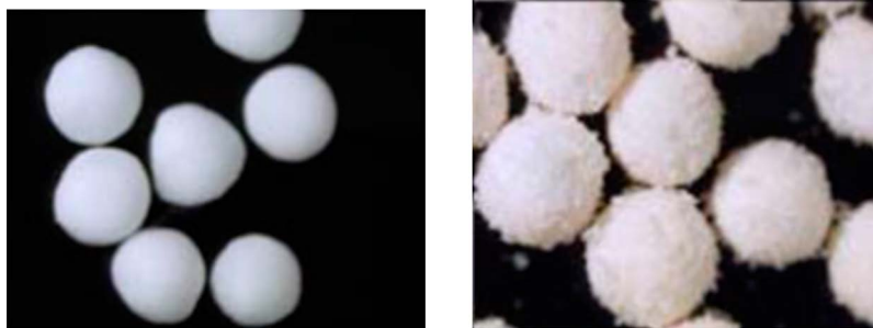
Figure 8.18 Images of uncoated seed particles ( left ) and dry powder-layered pellets ( right ). 33 Published with permission from Colorcon.
