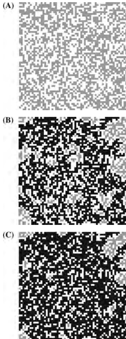
Figure 2 The basic percolation problem (for clarity, the percolating cluster is shown in black and nonpercolating clusters in gray). (A) p < p_c (B) p = p_c (C) p > p_c .
