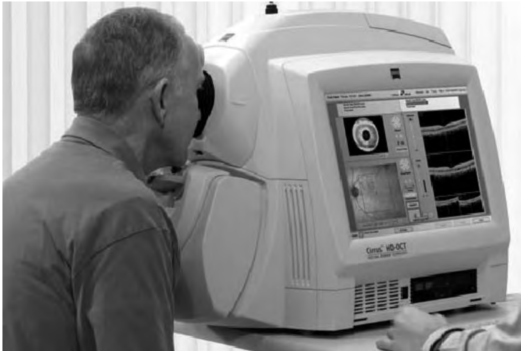
Figure 1 The Cirrus HD-OCT high-definition optical coherence tomography instrument, Carl Zeiss Meditec AG, is capable of feature resolutions in ocular tissue on the order of 5 to 25 \mu\text{m} .
