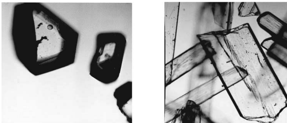
Figure 5 Photomicrographs showing well-defined crystals of famotidine with form A adopting an isometric prismatic morphology ( left ) and form B a platy morphology ( right ).
