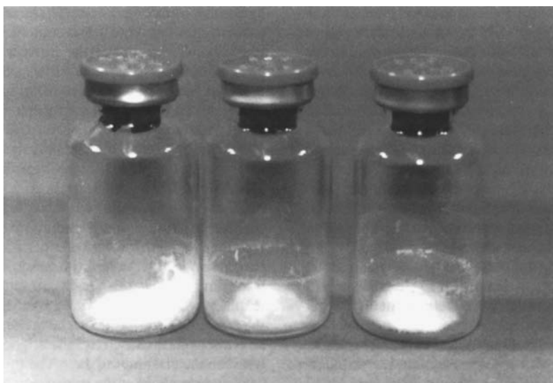
Figure 7 Collapse is characteristic of amorphous materials and can occur either during the freeze-dry process or during storage.
