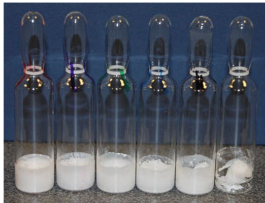
Fig. 10 Freeze-dried appearance of influenza antigen excipients (from left to right: 1%, 1.2%, 1.4%, 1.6%, 1.8%, and 2.0% sucrose in PBS). Increasing the sucrose above 1.4% resulted in progressively unacceptable freeze-dried product appearance when using the same FD cycle
