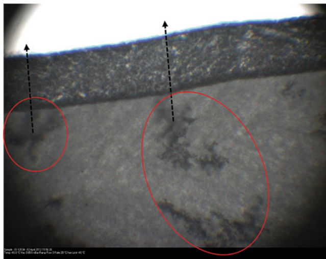
Fig. 8 FDM image of a co-solvent-based formulation following freezing and the application of vacuum, showing evidence of egress of the (more volatile) organic solvent from certain areas (examples highlighted by red circles, with direction of solvent vapor movement indicated by dashed arrows)
