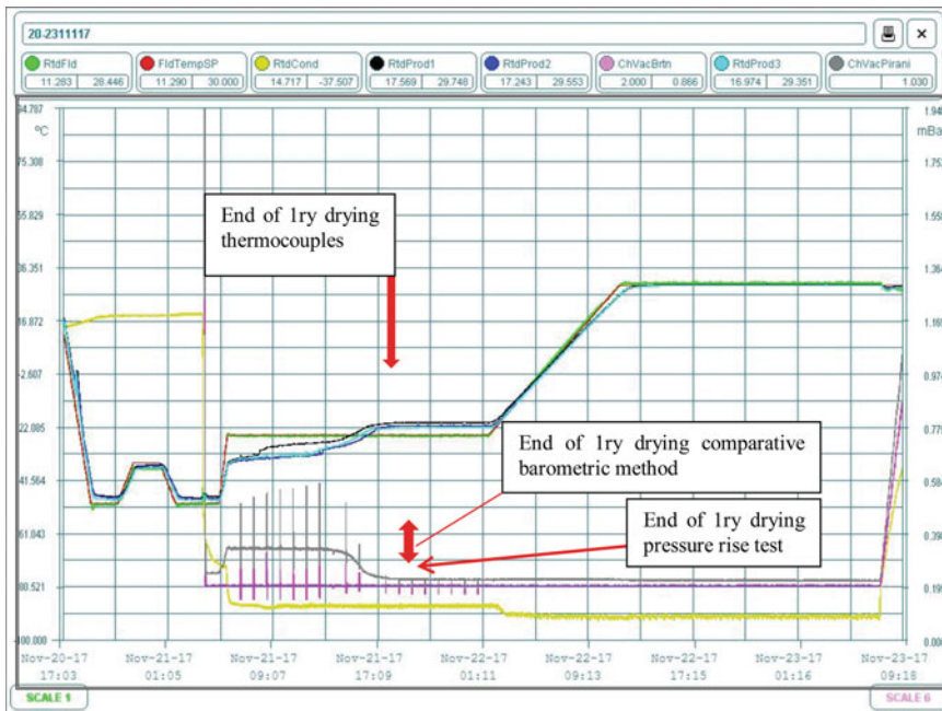
Fig. 14 Cycle optimization—endpoint determination methods on whole batch (pressure rise and comparative barometric readings) and individual probes (thermocouple) both indicating that the primary drying step in this cycle could be reduced in length significantly without impacting the end of this stage of drying (x axis time, y1 axis temperature(oC), y2 axis vacuum (mBar))
