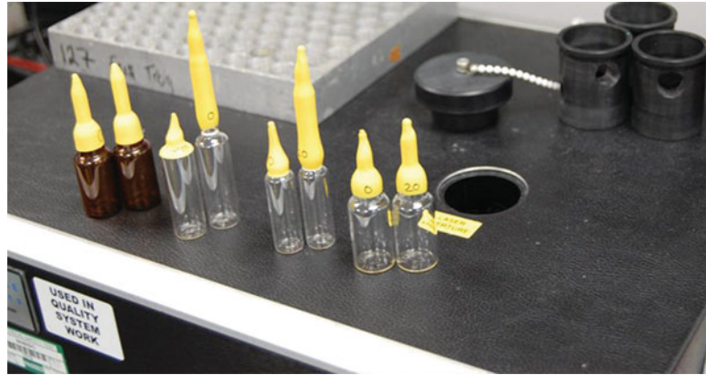
Fig. 6 Noninvasive oxygen headspace determination (FMS 760 Lighthouse Instruments, Charlottesville, VA, USA), calibrated using NIST-traceable oxygen standards in identical format containers
