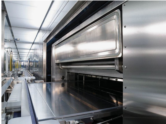
Fig. 1 A loading and unloading door, including a connection plate to a loading and unloading system
