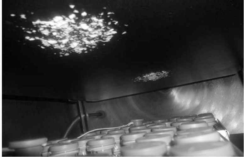
Fig. 4 Blow-out coating the upper shelf observed when freeze-drying 0.9% saline
