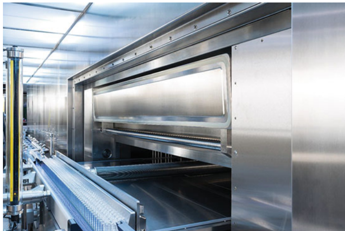
Fig. 7 A stationary push-push ALUS™ (back-pusher system)
