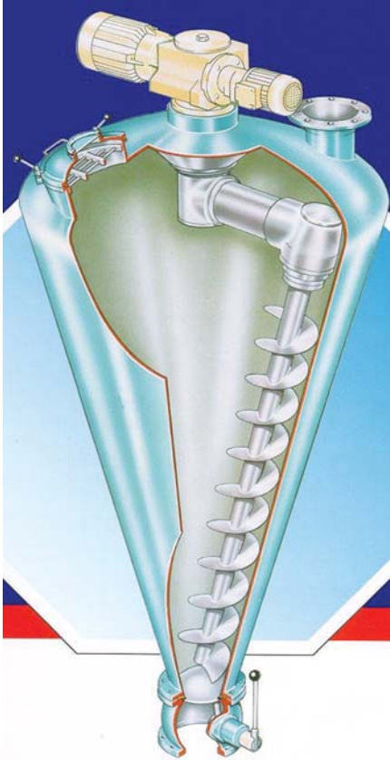
FIGURE 13.14 Conical screw mixer. (Vrieco-Nauta; courtesy of Hosokawa Micron Powder Systems.)
