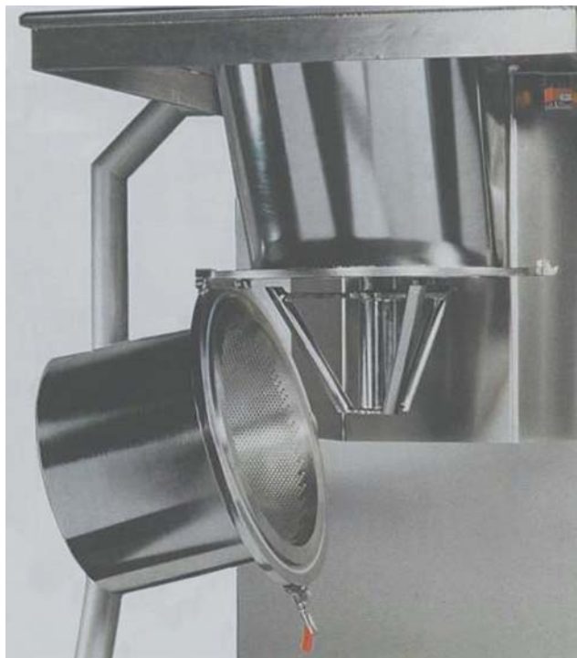
FIGURE 13.8 Cone mill blade configuration. (Courtesy of Hosokawa Micron Powder Systems.)
