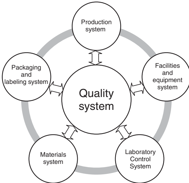
FIGURE 29.2 Six-system inspection model (From FDA, 2006.)
