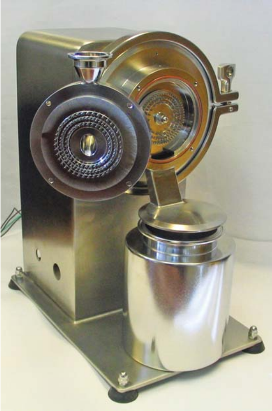
FIGURE 13.10 Pin mill. (Courtesy of Hosokawa Micron Powder Systems.)
