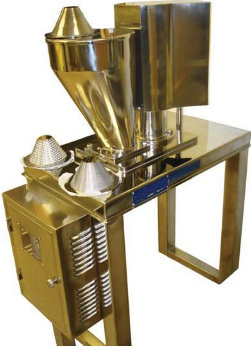
FIGURE 13.7 Cone mill. (Courtesy of Mendel Corporation.)
