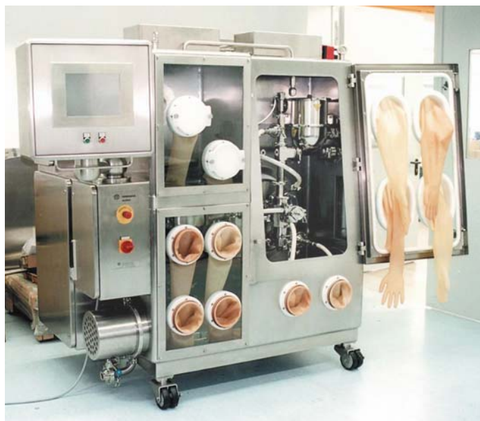
FIGURE 13.12 Fluid energy mill in self-contained clean-in-place isolator. (Courtesy of Hosokawa Micron Powder Systems.)
