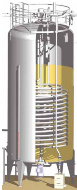
Figure 3.9 Large-scale acetator for the production of vinegar used in most modern facilities (with kind permission from FRINGS brochure).
