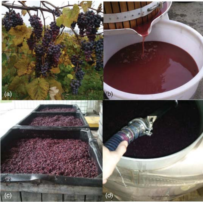
Figure 3.8 Important aspects of wine making. Different varieties of grapes are used for white (Riesling, chardonnay, and sauvignon blanc) and red wines (merlot, pinot noir, and shiraz; (a)). The crushing, pressing (b), and pretreatment are different for white and red wines. For red wines, the juice and skins are fermented together (c). The skins float, and the juice is pumped over (d) the skins to extract color (because of the red and purple anthocyanins) and phenolics such as tannin.
