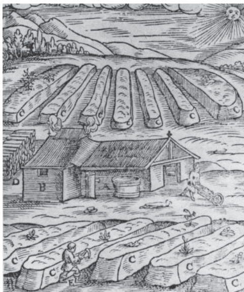
Figure 1.3 Saltpeter manufacture toward the end of the middle ages. Heaps of earth, soaked with animal and human excrements and blood were aerated with picks and rakes. The ammonium (and ammonia, respectively) released from the nitrogen-containing organic matter was oxidized by aerobic nitrifying bacteria to nitrate ( \text{NO}_3^- ). Nitrate then was leached out as potassium or sodium nitrate. The depleted soil was recovered and recycled. Source: Reproduced from “Berg- und Probirbuch” by Lazarus Erker (1574).
