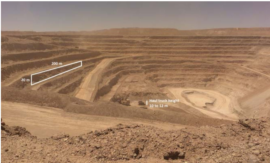
Figure 13.6 Open-pit copper mine in northern Chile. The terrace height is 20–25 m. Also note the haul truck in the middle as a size reference. Source: Photograph by Sören Bellenberg.
