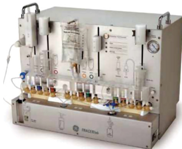
Figure 13.3 Early TRACERlab MX FDG cassette-based synthesis module. Source: Image courtesy of GE.
