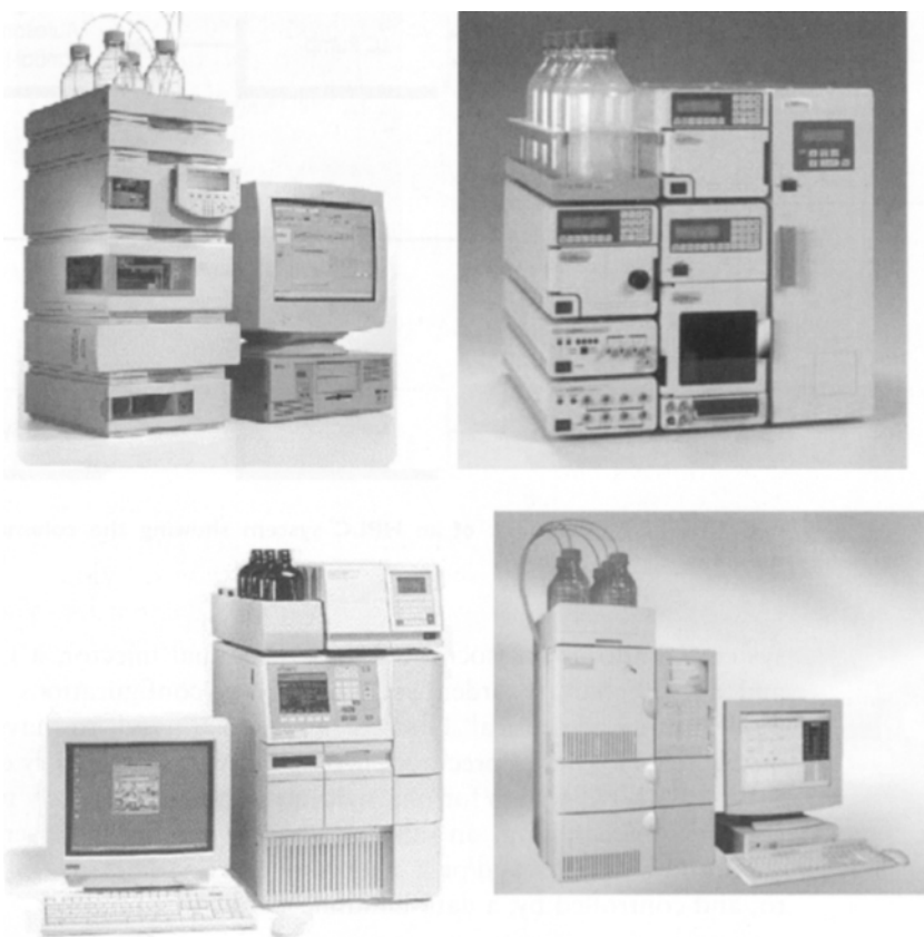
FIGURE 2 Examples of modular and integrated HPLC systems. Upper row (l to r) modular systems: Agilent 1100 Series, Jasco LC-2000 Series; Lower row (l to r) integrated systems: Waters Alliance, Shimadzu LC-2010.
