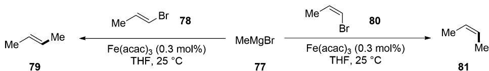
Fig. 17 Maintenance of E,Z -stereochemistry in vinylation of MeMgBr
