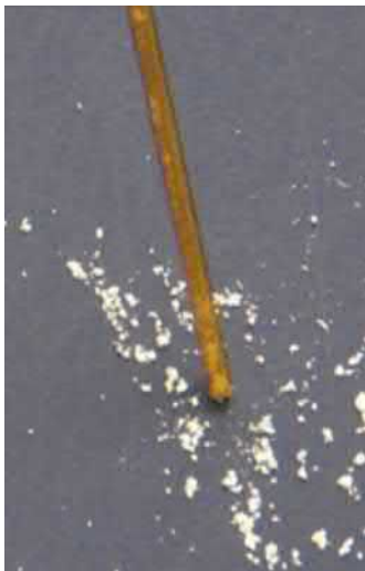
FIGURE 4.1 Example of solid particles eluting from an unstable PLOT column.
