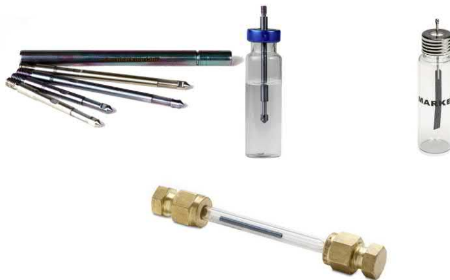
FIGURE 10.19 Sorptive devices compatible with direct immersive sampling. Clockwise from top left: HiSorb, thin-film SPME and SPE-tD.
