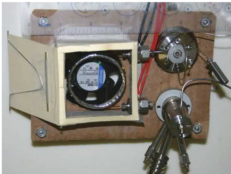
FIGURE 17.25 A second prototype portable GC with a diaphragm valve, micro PDD, and resistance heated column. Courtesy of Valco Instruments.
