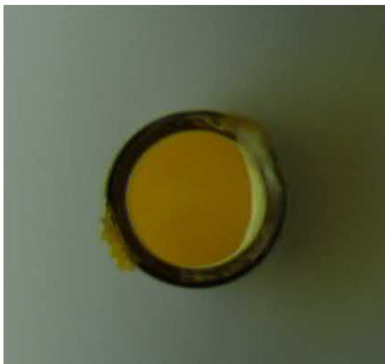
FIGURE 4.6 Cross view of a crescent PLOT column after spin coating for 60 min at 3500 rpm.
