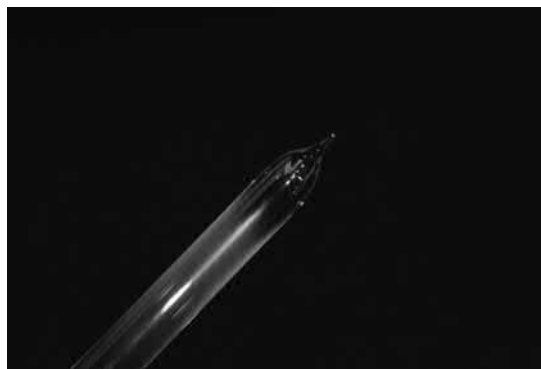
FIGURE 3.1 Neck down area on a fused-silica preform.
