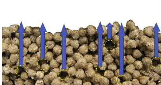
FIGURE 4.2 Schematics of a PLOT column particle-based layer where “pockets” are present.
