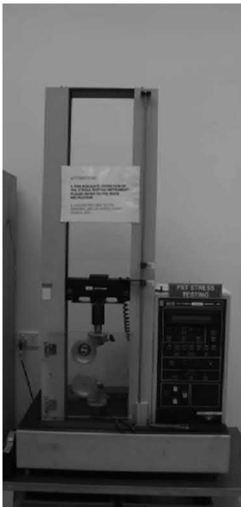
FIGURE 3.6 Tensile testing of capillaries.
