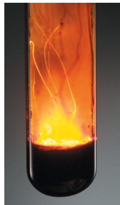
▲ Figure 1.8 The reaction of aluminum with bromine releases energy in the form of heat.
