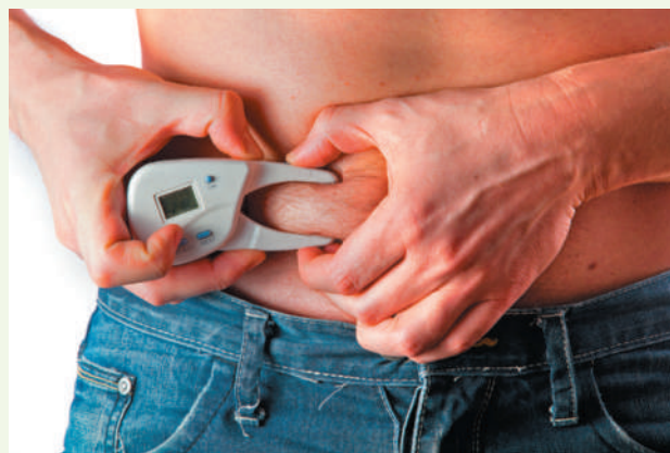
▲ A person's percentage body fat can be estimated by measuring the thickness of the fat layer under the skin.
