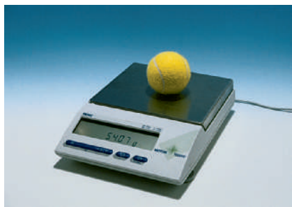
▲ The tennis ball weighs 54.07 g on this common laboratory balance, which is capable of determining mass to about 0.01 g.
