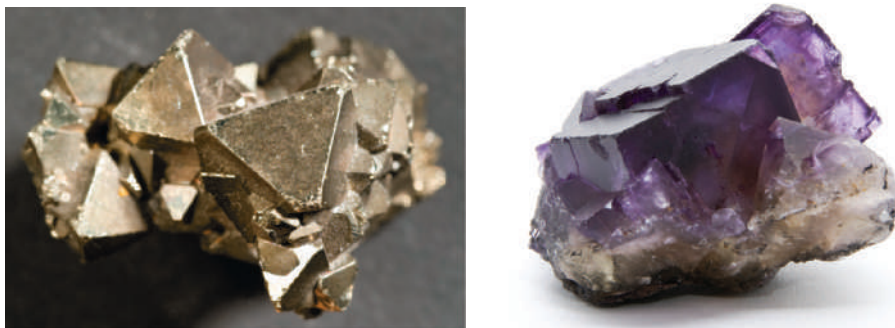
▲ Crystalline solids, such as pyrite (left) and fluorite (right), have flat faces and distinct angles. The octahedral shape of pyrite and the cubic shape of fluorite reflect similarly ordered arrangements of particles at the atomic level.
