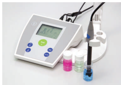
▲ Figure 10.3 Using a pH meter to obtain an accurate reading of pH.
