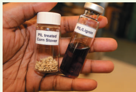
▲ Protic ionic liquids (PIL) are used to extract lignin from biomass (right) leaving behind the solid, energy-rich cellulose (left) to be converted into biofuels.
