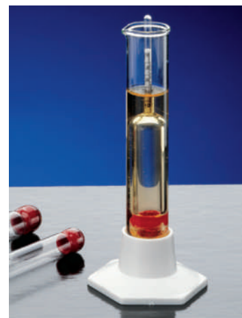
▲ The specific gravity of urine, measured by a urinometer, is used to diagnose conditions such as diabetes.
