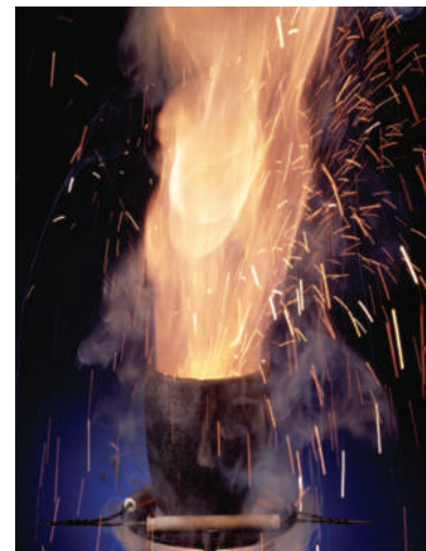
▲ The reaction between aluminum metal and iron(III) oxide, called the thermite reaction , is so strongly exothermic that it melts iron.
