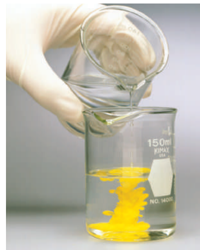
▲ Reaction of aqueous Pb(NO 3 ) 2 with aqueous KI gives a yellow precipitate of PbI 2 .
