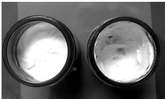
Figure 13.9 A well combined cream (left) – all the ingredients are combined homogeneously, creating a smooth cream – and a poorly combined cream (right) – note the splitting (separation) of the constituents.
