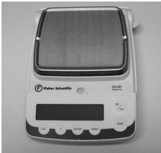
Figure 13.2 A top-pan balance used for measuring more than 10 grams of an ingredient.
