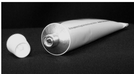
Figure 11.5 A tamper-evident seal; the metal container around the product is continuous until first administration by the patient, who breaks the seal using the point inside the cap.
