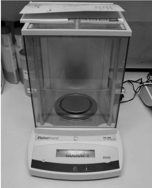
Figure 13.1 A Class B balance used for weighing small quantities of powders.
