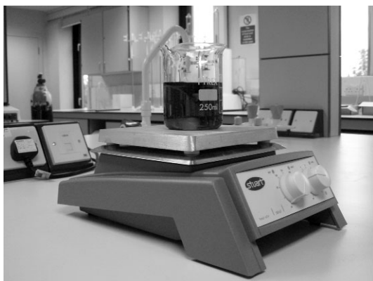
Figure 13.12 An electric hot plate with magnetic flea (stirrer), which allows for constant gentle stirring.
