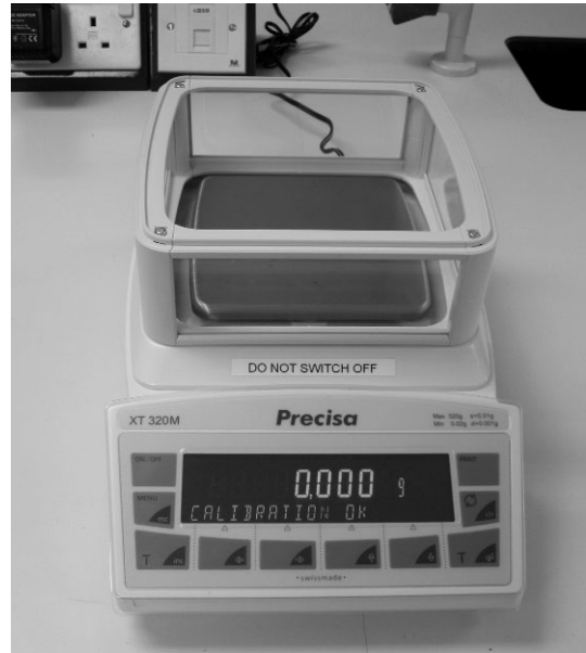
Figure 13.3 A Class I balance used to measure less than 10 grams of an ingredient.
