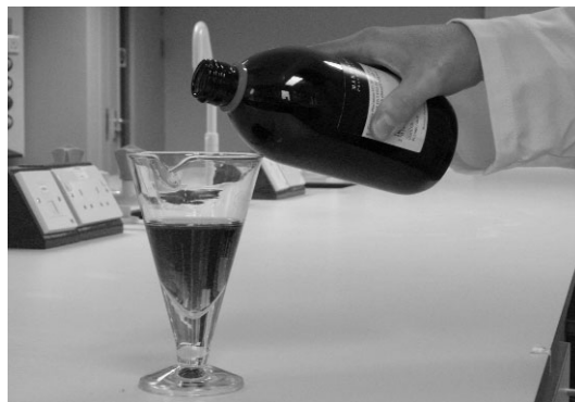
Figure 13.6 Correct pouring technique: protecting the label from spillage or drips.
