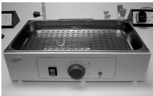
Figure 13.11 A water bath used for melting large quantities of solid ingredients.
