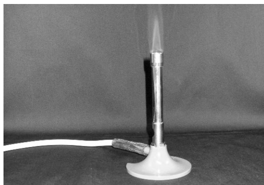
Figure 13.10 A Bunsen burner. In the 'on' position it has a blue flame and in the 'standby' position it has a highly visible orange flame.
