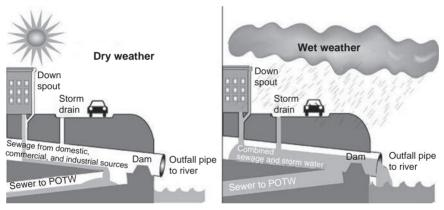
Figure 5.21. Combined sewer overflow
