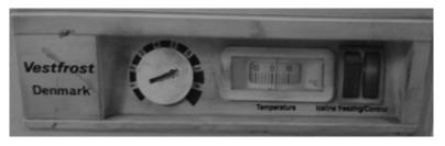
Figure 9.8. The temperature reader of an ILR
