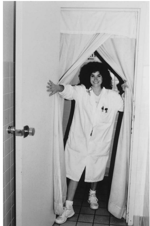
FIGURE 48.2 AIDL insectary. Overlapping cloth sheets stapled across internal door to dislodge mosquito escapees from clothing.
