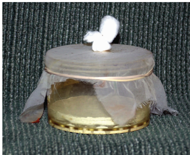
FIGURE 56.1 Container for oviposition, larval rearing, and adult emergence of phlebotomine sand flies. The plastic container is 12 cm in diameter, with holes drilled in its bottom, and layered with 1.5 cm of plaster of Paris. Fine mesh over the top is held in place tightly with a rubber band. A cotton plug in the mesh opening permits admission or removal of adults with the aspirator shown in Figure 56.2. Photo by L. E. Munstermann.
