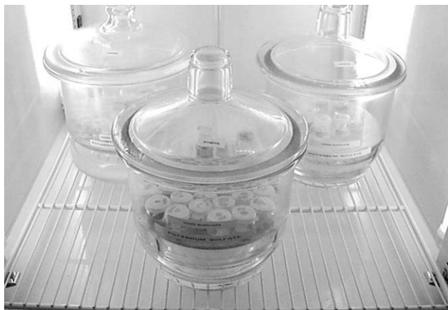
FIGURE 49.6 Glass dessiccators within a temperature- and light/dark-cycle-controlled environmental chamber used to house tick colonies. The dessiccators basins should contain saturated salt solutions to maintain sufficient humidity, critical to the ticks' viability (see text). Photo courtesy Ken Bourell.
