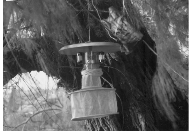
FIGURE 19.9 CDC light trap of Sudia and Chamberlain (1962). Photo by C. G. Moore, CDC.
