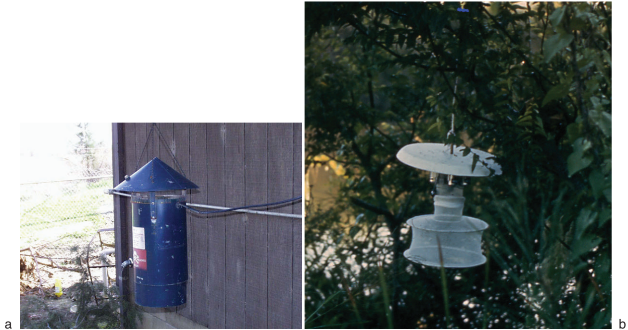
FIGURE 9.16 Traps used to sample adult mosquitoes: (a) Standard New Jersey light trap; (b) CO 2 -baited CDC-style trap. (a) Courtesy of Sacramento-Yolo Mosquito and Vector Control District; (b) photograph by Bruce Eldridge.
