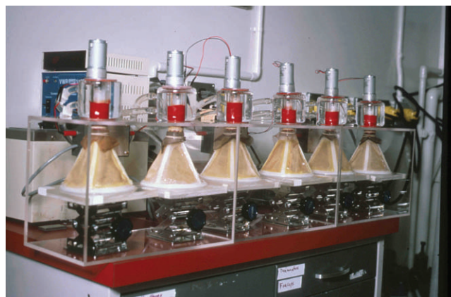
FIGURE 54.1 Female Culicoides sonorensis (located inside insect-secured blood-feeding cones) feeding on sheep blood contained inside an artificial blood-feeding apparatus. (Note: Insects feeding on BSL-3 infectious bloods would require the feeding apparatus to be operated within a biological safety cabinet.)
