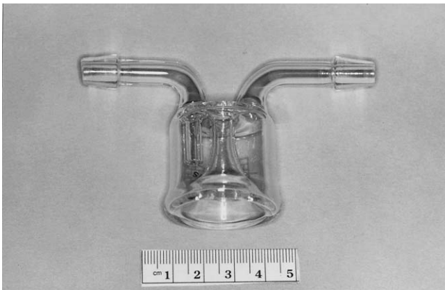
FIGURE 53.6 Detail of glass feeder. Water is pumped into the feeder's water jacket via the left inlet tube and exits via the right outlet tube.
