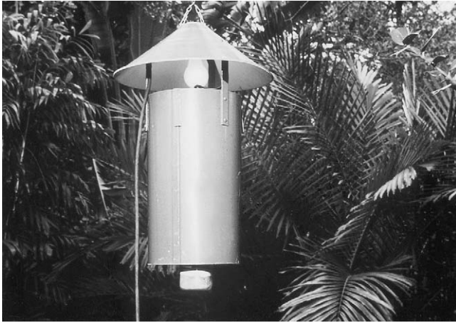
FIGURE 19.8 New Jersey (or Mulhern) light trap. CDC file photo.
