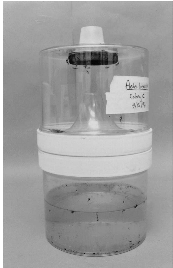
FIGURE 53.4 Mosquito breeder (BioQuip Products). Mosquitoes emerge from pupae held in the lower chamber and fly upward for easy isolation in the upper chamber.
