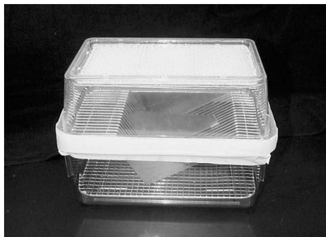
FIGURE 49.2 Conventional shoebox-style mouse cage with wire-rack bottom used for housing mice during infestation with larvae or nymphs. The cage must be taped along the junction between bottom and lid to prevent tick escape. Photo courtesy Ken Bourell.
