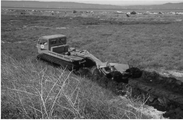
FIGURE 9.20 Ditching of salt marsh to improve natural tidal flushing action for reduction of mosquito populations. Courtesy of Alameda County (California) Mosquito Control District.
