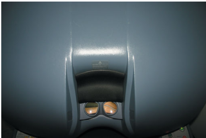
Figure 19.4 da Vinci console – binocular viewer (photo courtesy of Daniel Leff).
