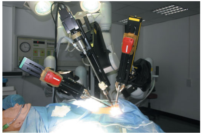
Figure 19.5 Slave unit: da Vinci arms set-up in a virtual operating theatre (photo courtesy of Daniel Leff).
