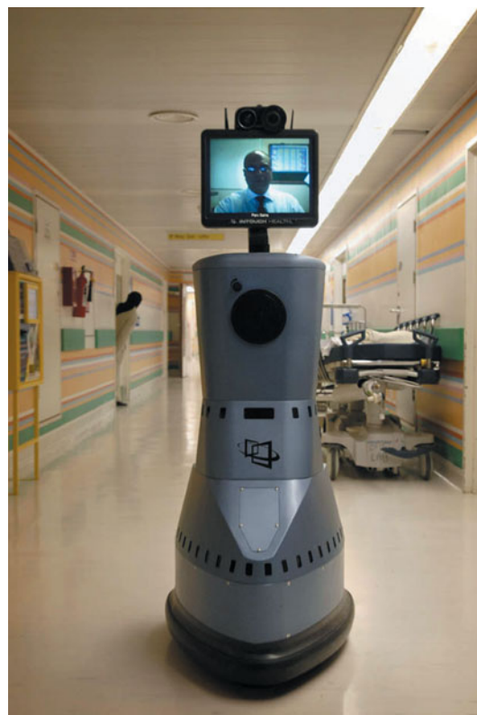
Figure 19.11 Remote presence robot (courtesy of the Department of Biosurgery and Surgical Technology, Imperial College, London).
