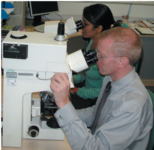
Figure 12.8 A double-headed microscope allows a histopathologist and a trainee to view a slide simultaneously.
