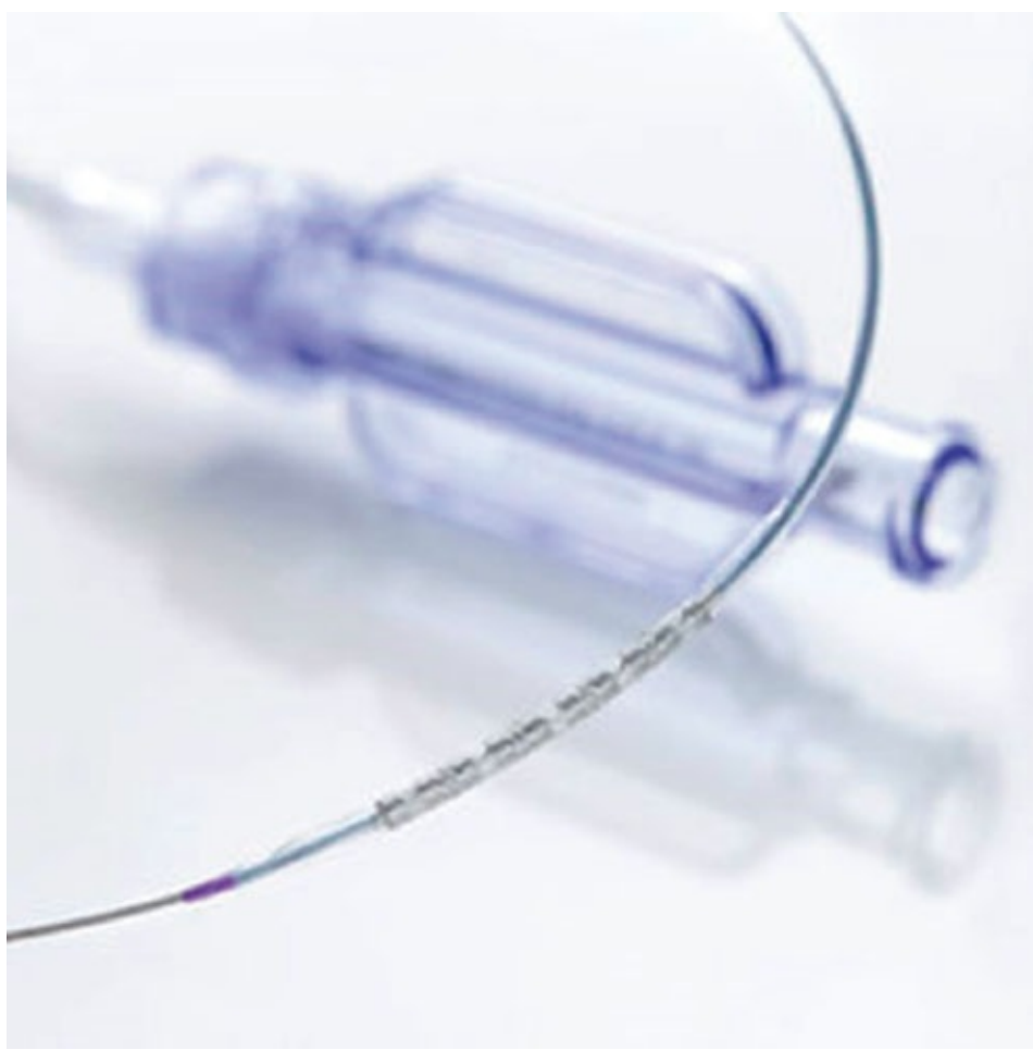
FIGURE 2.17 GRAFTMASTER RX stent (Abbott Vascular). The GRAFTMASTER RX stent has replaced the original “JOSTENT,” and it is indicated for the treatment of free perforations in native coronary vessels or saphenous vein bypass grafts \geq 2.75 mm in diameter. It consists of an ultrathin PTFE expandable layer sandwiched between 2 coaxial 316L stainless steel, slotted-tube, balloon-expandable stents. It is available in 6F compatible sizes with a diameter of 2.8, 3.5 and 4.0 mm, and 7F compatible sizes with a diameter of 4.5 and 4.8 mm. Courtesy of Abbott Laboratories. 100 Abbott Park Road. Abbott Park, Illinois 60064–350.
