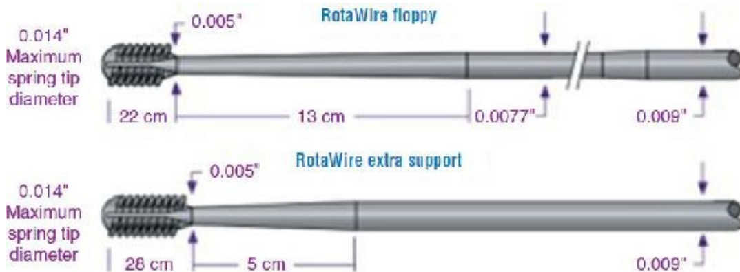
FIGURE 19.5 Rotational atherectomy. The RotaWires are designed specifically for the use with the rotational atherectomy system. They are made of a 0.009" stainless steel core with tapered distal ends for varying degrees of burr support. A 0.014" distal platinum coil prevents the burr from traveling beyond the tip of the wire. Image provided courtesy of Boston Scientific. ©2018 Boston Scientific Corporation or its affiliates. All rights reserved.
