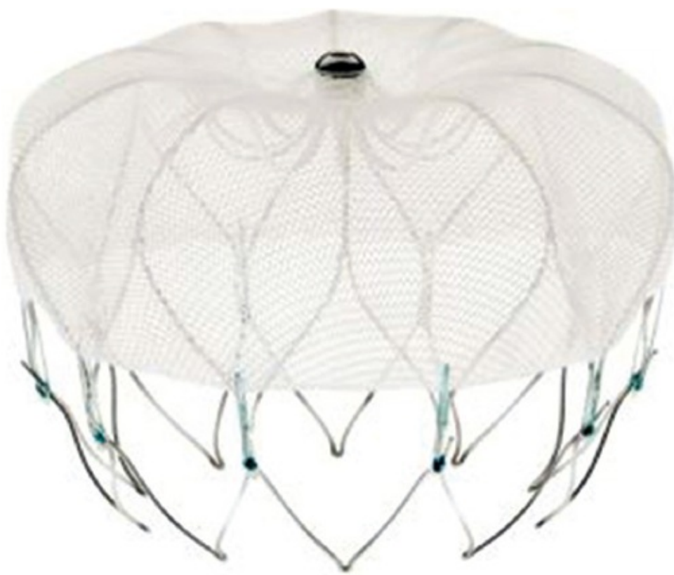
FIGURE 22.19 The WATCHMAN Device. The WATCHMAN Device is made of a nitinol frame that radially expands to maintain position in the LAA and has 10 active fixation anchors to engage the LAA tissue. A 160-micron polyethylene terephthalate cap is designed to block emboli from exiting the LAA and promote healing.
