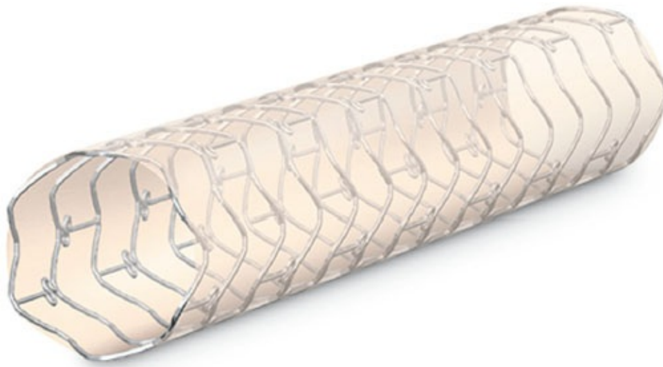
FIGURE 2.18 Aneugraft Dx (Amnis Therapeutics). The Aneugraft Dx is a single-layer coronary stent graft covered by equine pericardium. It consists of a 316L stainless steel metal stent covered by an equine pericardium cylinder. The bovine pericardium is sutured on the bare metal stent with a propylene suture. It is a low-profile stent that can be delivered through a 6F guiding catheter. Courtesy of Amnis Therapeutics Ltd., 22 Ha'ilan Street, P.O. Box 146, Or Akiva, 3060000 Israel. info@amnis.life .
