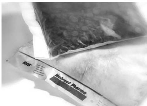
Figure 11 Picture of a ready-for-sterilization bag. The bag on the bottom has its Tyvek side up; the bag on top has its non-Tyvek side up.
