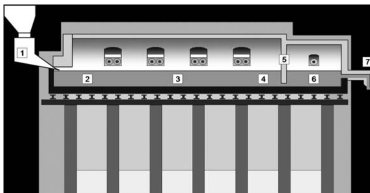
Figure 5 Longitudinal cross section of a large industrial glass melting furnace. Raw materials are added continuously at the batch feeder (1). Melting (2), refining (3), and homogenization (4) occur gradually as the melt progresses through the main furnace chamber. The molten glass flows under the bridge wall (5) into the conditioning section (6) before passing into the forehearth (7) for transfer to the blow-molding or tube draw process. Source: From Ref. 2.
