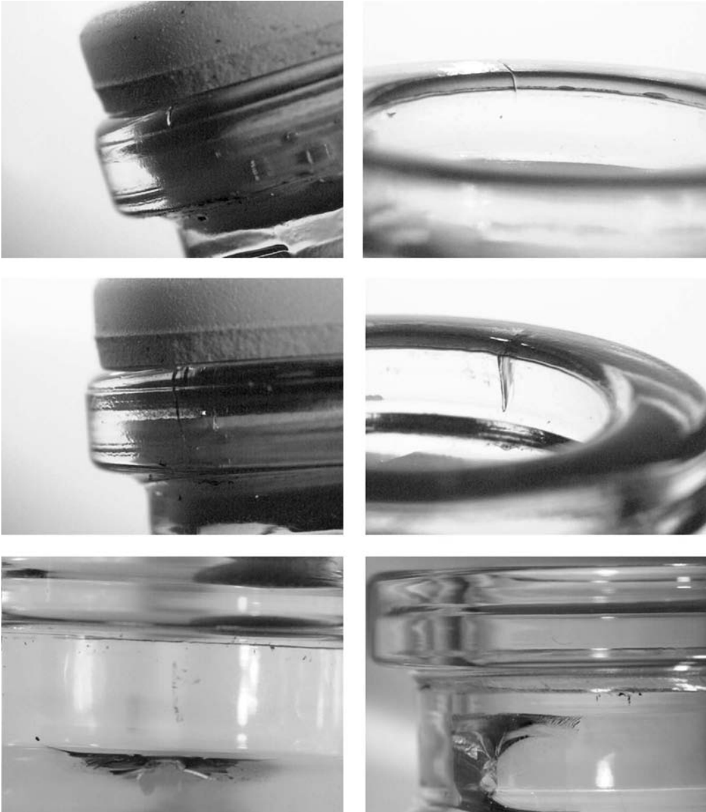
Figure 8 Defects found in glass vials. Top row: Line-over defect likely created during vial manufacturing process. Middle row: Crack in vial finish likely created during vial manufacturing or distribution to end-user. Bottom row: Crack in vial shoulder ( left ) and vial neck ( right ) likely created at the end-user manufacturing site. Source: Anonymous upon request.
