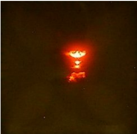
Figure 11(a). Plasma generated on the phosphor screen as high emission current impacts on the screen causing gases release into the surrounding vacuum.
