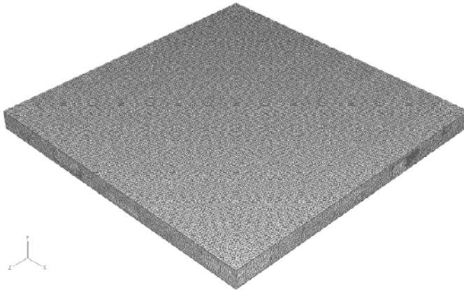
Figure 28. Meshed Unit Cell using a total of 1,300,955 DC3D4 elements.
