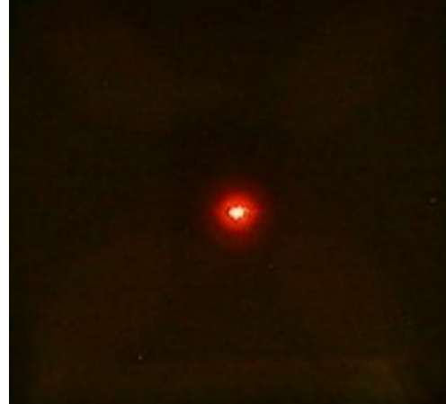
Figure 11(b). Field emission electrons from one pixel of field emitter array hit the phosphor screen and generate bright illumination.
