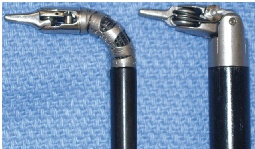
Fig. 2.14 Photograph of Endowrist® needle drivers. On the left is a 5-mm needle driver with the “snake joint” compared to the 8-mm needle driver with an “angled joint”
