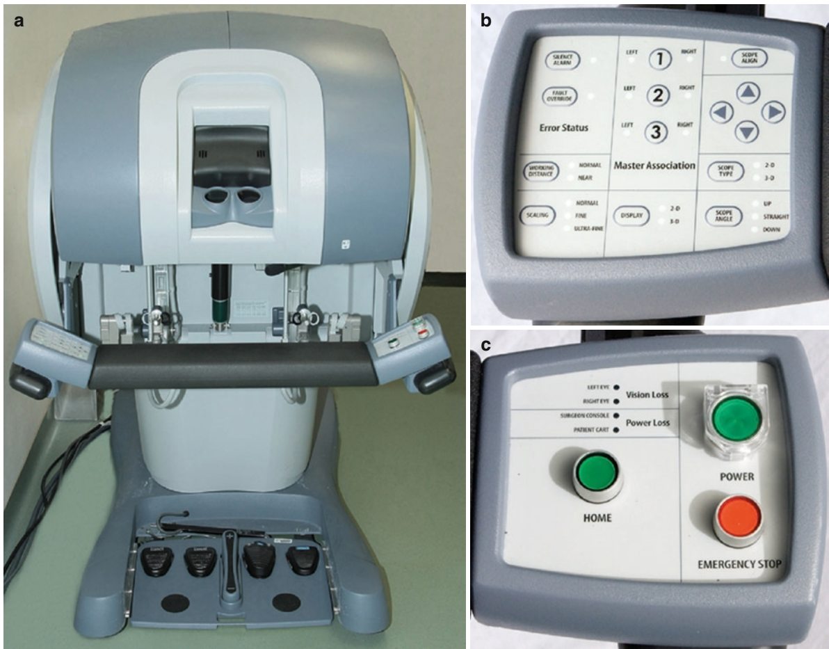
Fig. 2.9 Photograph of da Vinci ® S surgeon console (a), left-side (b), and right-side (c) pod controls
