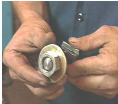
Figure 2. Use a bolt that does not require more than two washers.
