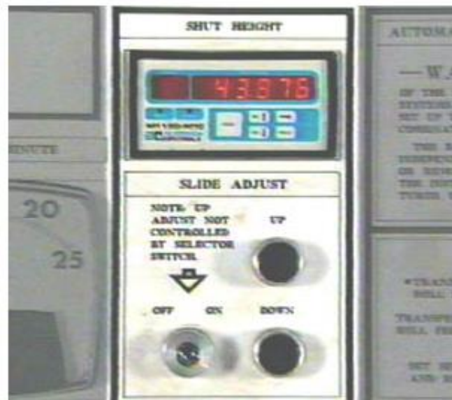
Figure 1. Press the slide adjust buttons to electrically adjust shut height.
