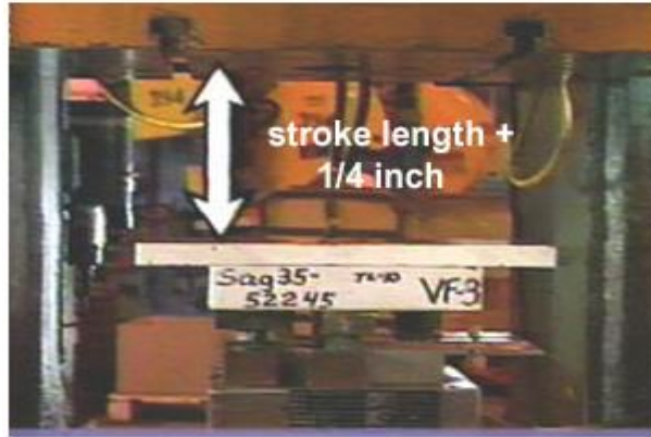
Figure 2. Proper shut height should be at least the stroke length plus 1/4 inch.
