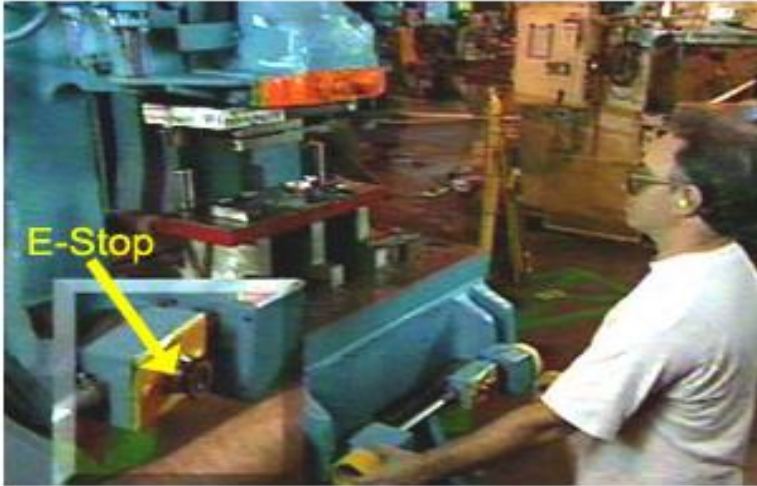
Figure 2. On full-revolution clutch presses, the E-stop button stops the main motor, but the ram does not stop until it returns to stroke-up position.
