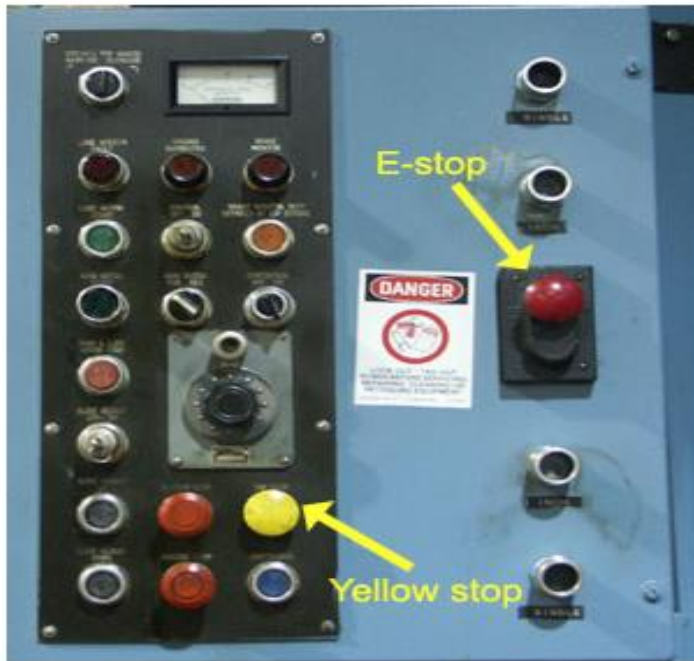
Figure 1. The E-stop button stops the press stroke immediately, and the yellow stop stops the press in the stroke-up position.
