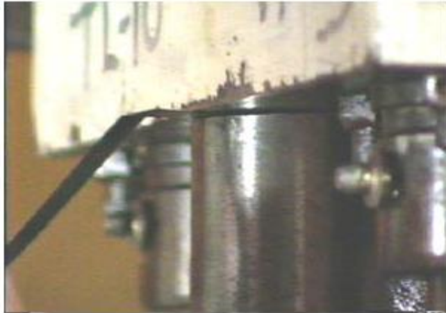
Figure 1. A feeler gauge determines if there is enough clearance between punch and die components.
