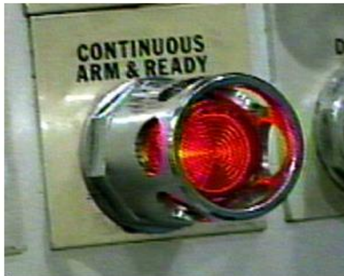
Figure 2. The arm control button prevents inadvertent startup of the press in continuous mode.
