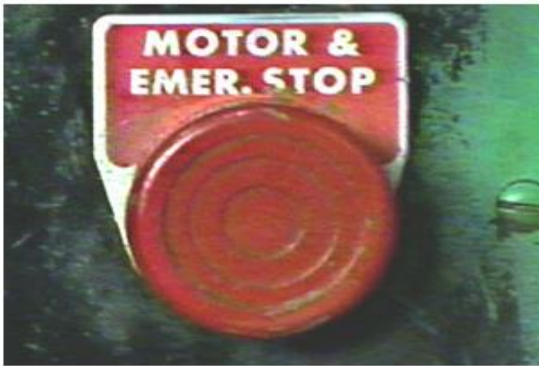
Figure 3. Some presses use the E-stop button as the main motor stop.
