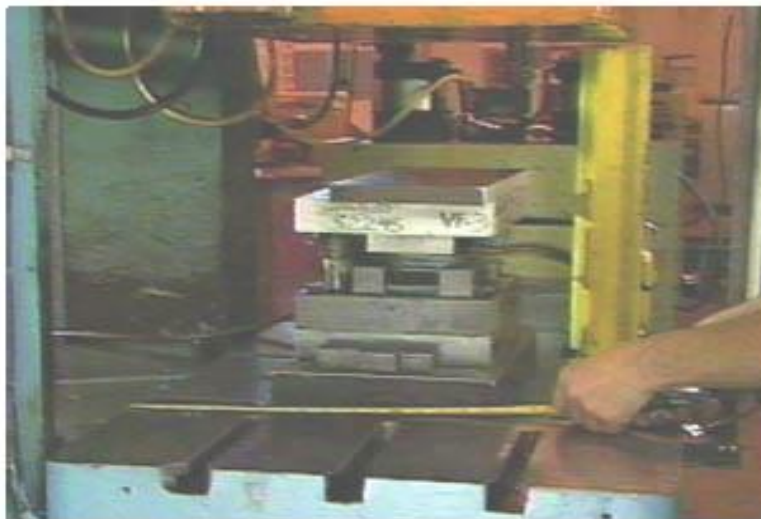
Figure 2. Take a measurement from the front to the back of the bolster.
