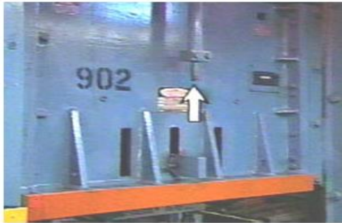
Figure 1. After installing a new die, you must readjust the knockout bar.
