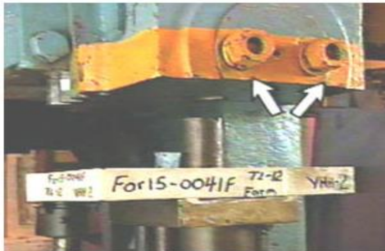
Figure 2. Tighten the shank locknuts to lock in the slide height.
