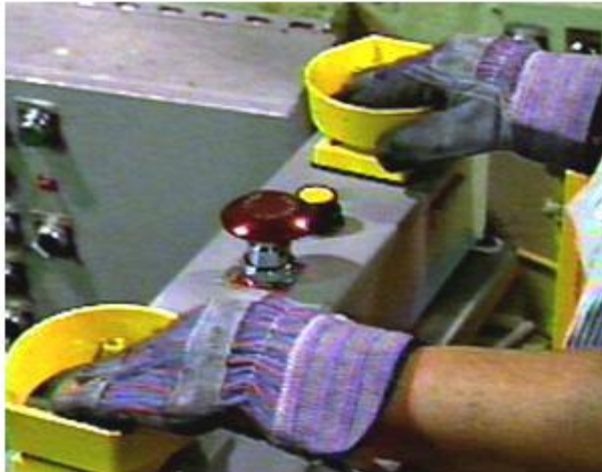
Figure 1. The press operator uses both hands to push the dual palm buttons at the same time.
