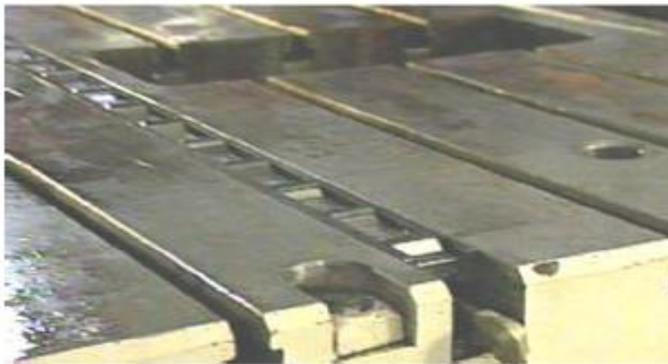
Figure 2. Die lifters should be all the way up so that the new die fits easily into place.
