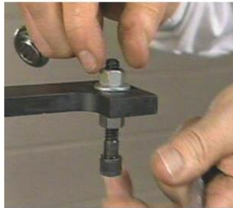
Figure 2. To move the arm of the striker out of the way, loosen the locknuts.
