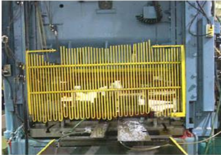
Figure 2. A barrier guard may signal the press to stop.
