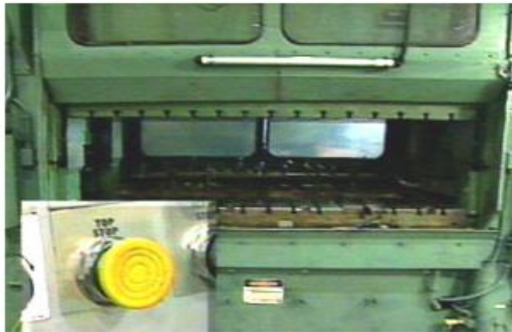
Figure 1. The yellow "top stop" button stops the press in the stroke-up position.
