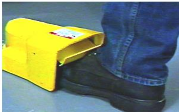
Figure 2. The press operator also uses a foot switch to initiate ram motion.
