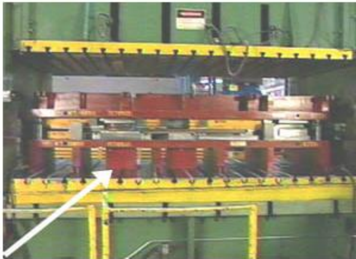
Figure 1. The die shapes and forms metal.
