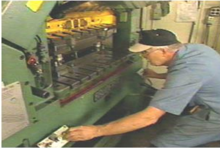
Figure 1. Inch the press through a stroke with nothing in the dies.
