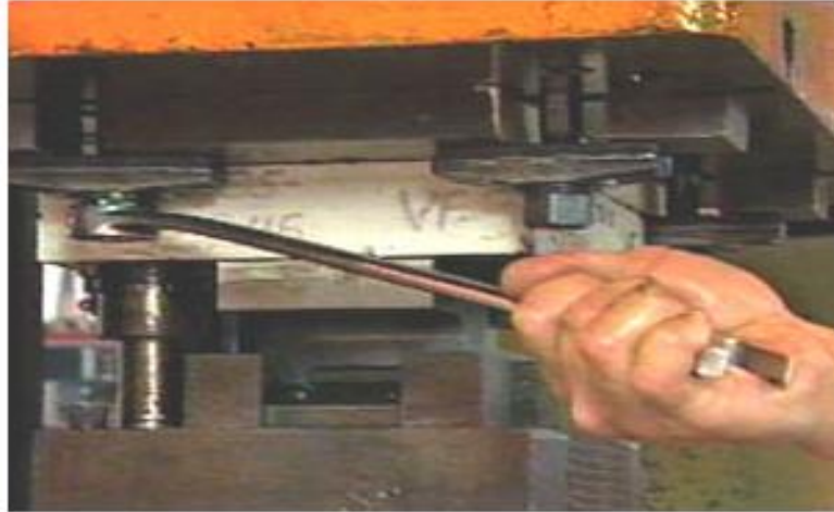
Figure 2. Alternate between tightening nuts on either side of the slide face.
