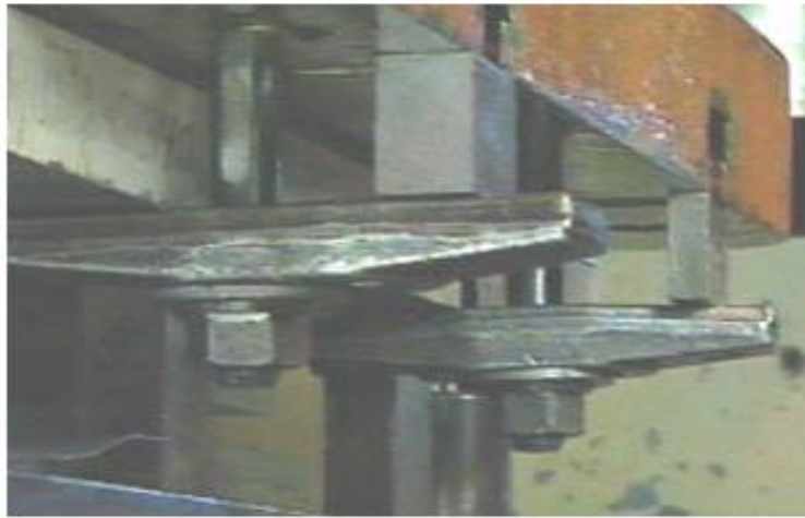
Figure 1. First, clamp the upper clamps to the face of the slide.
