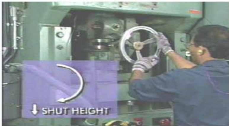
Figure 3. Turn the adjusting screw either clockwise or counterclockwise when using a gear-driven slide adjuster.
