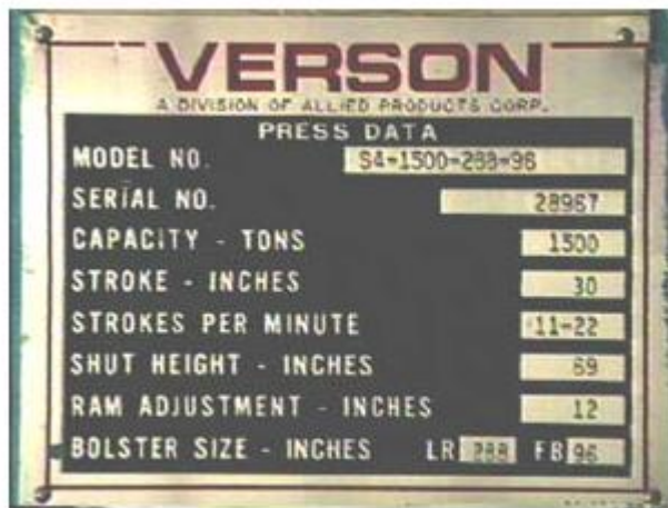
Figure 1. The press specification plate identifies important information for die changing.
