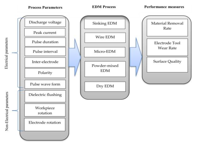
Figure 1. Electric discharge machining (EDM) processes, process parameters and performance measures.
