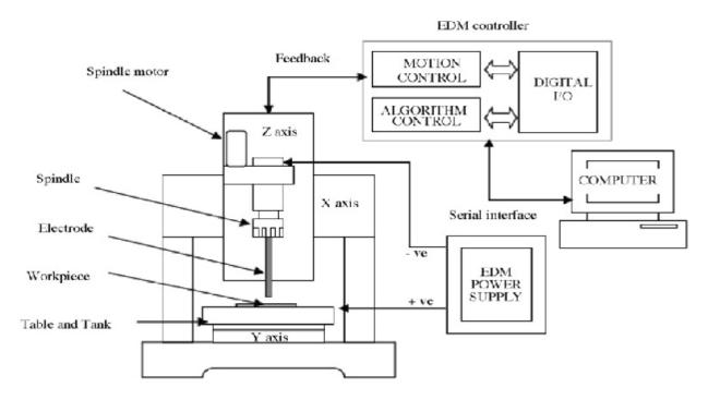
Schematic diagram of micro-EDM
