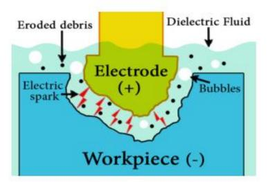
Figure 2. Principle of EDM.
