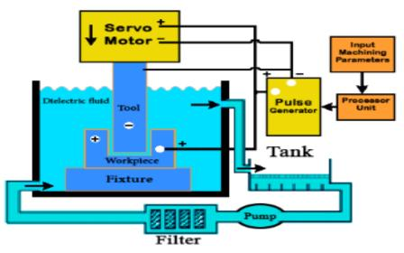
Figure 3. Schematic diagram of the die-sinking EDM.
