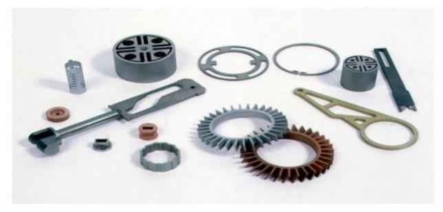
Figure 3: Difficult internal parts made by EDM process
