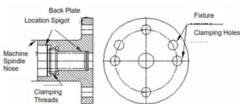
Figure 4.7 : Back Plate for Turning Fixture
