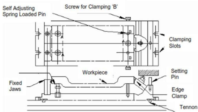
Figure 4.4 : Face Milling Fixture
