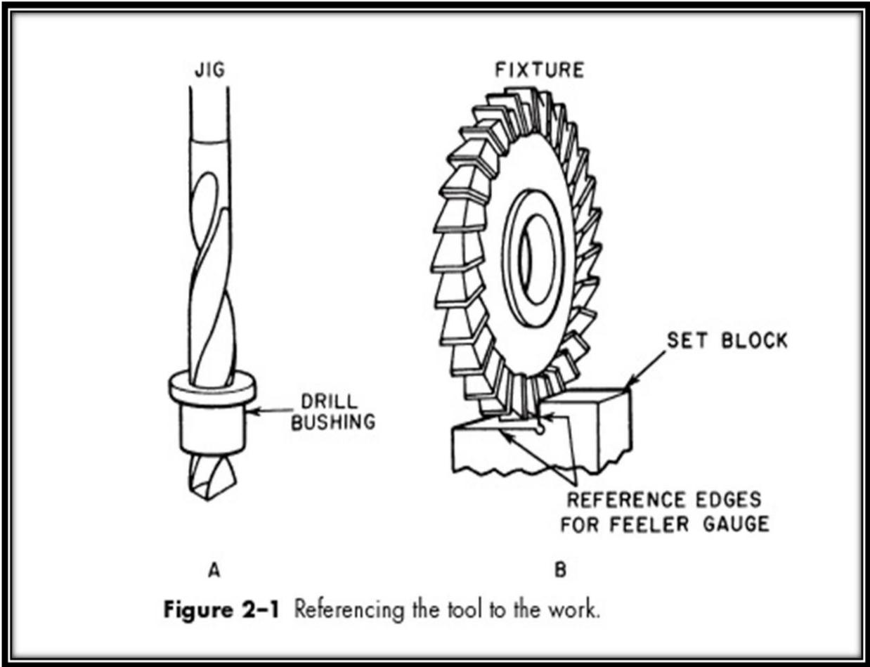
**Figure 2-1** Referencing the tool to the work.
