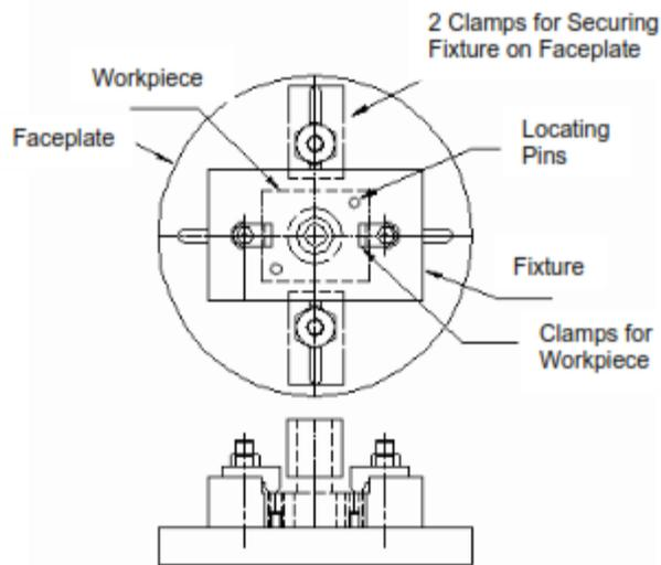
**Figure 4.5 : Face Plate Fixture**
