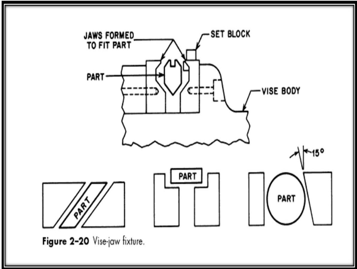
Figure 2-20 Vise-jaw fixture.
