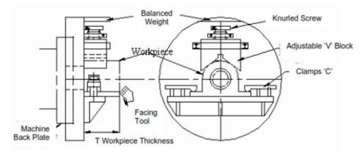
Figure 4.6 : Turning Fixture (Boring and Facing Fixture)
