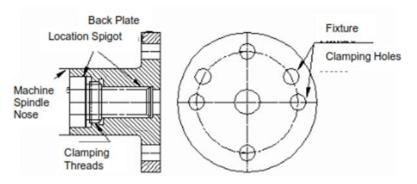
Figure 4.7 : Back Plate for Turning Fixture
