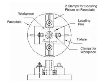
Figure 4.5 : Face Plate Fixture
