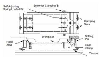
Figure 4.4 : Face Milling Fixture
