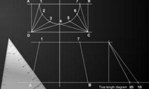
Step 9, Mark a point on the base line to the right of point 1D
