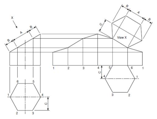
Figure2: Development of hexagonal prism and truncated hexagonal prism
