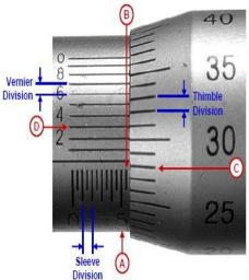
How to read a vernier metric micrometer: Sleeve div. = 1 mm Thimble div. = 1/50<sup>th</sup> of sleeve sub-div. = 1/100 mm Vernier div. = 1/10<sup>th</sup> of thimble div. = 1/1000 mm A. The highest figure: 5 \* (sleeve div.) = 5 mm B. The half-figures: 1 \* (sleeve sub-div.) = 0.5 mm C. The highest figure: 28 \* (thimble div.) = 0.28 mm D. The matching figure: 3 \* (vernier div.) = 0.003 mm FINAL READING = A + B + C + D = 5.783 mm
