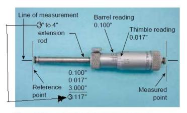
For example. to read Inch system inside micrometer; look at the figure below.
