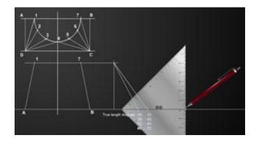
**Step 10**Set the compass at the distance between D and C on the top view (as this is already true length), then transfer the distance D to C to the base line. Label the points D and C. Reset the compass to the length of the line 4D. Placing one point on D, draw an arc midway between D and C. Shift the compass to C, draw an arc to bisect the previous one. Label this point 4.
