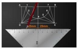
**Step 7**The base is 70mm square. Draw lines from the base to the top. Label the base points A and B. Label the top points 1 and 7.
