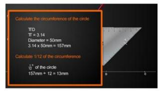
**Step 12**Measure and mark out 13mm on the reference line. Set the compass at 13mm (1/12th circumference).
