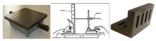
A surface gauge is used on surface plates for scribing lines on work pieces and checking parallel surfaces and heights.
