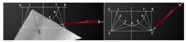
**Step 6**Draw the side view. First, draw a reference line. Remember, the vertical height is 50mm, and the diameter of the top is 50mm.
