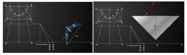
**Step 11**Mark out a new short reference line for 1/12th of the circumference of the top of the square to round shape.
