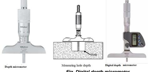
Fig. Digital depth micrometer
