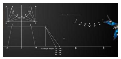
Step 13 Develop the half square base from point D to point A.
