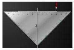
**Step 2**Develop the top view. With a set square, mark out the measurements for half the base, and label each corner (from the top left hand corner, moving clockwise) A to D.
