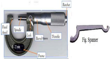
Fig. Parts of outside micrometer
