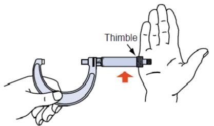
Figure. Roll the thimble on your hand for long spindle movements.
