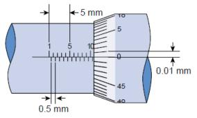
Fig. Metric Micrometer markings and graduations
