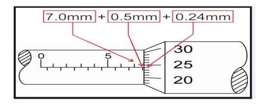
Example. 3 Reading outside micrometer with a range of 50 to 75 mm. (see figure bellow)
