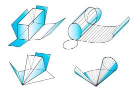
Many articles such as **cans**, **pipes**, **elbows**, **boxes**, etc. are manufactured from thin sheet materials. Generally a template is produced from an orthographic drawing when small quantities are required, and the **template** will include allowances for bending and seams, bearing in mind the thickness of material used.
