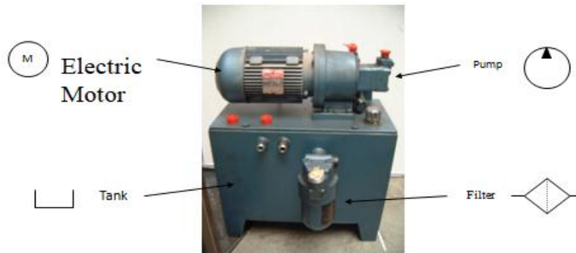
Figure3: hydraulic power pack
