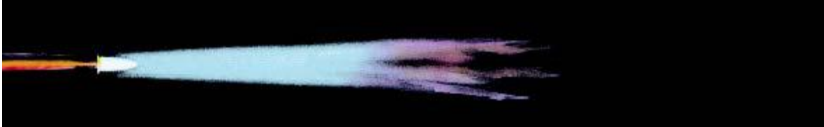
Figure 12. Oxidizing Flame (Acetylene and excess oxygen, 6300°F)
