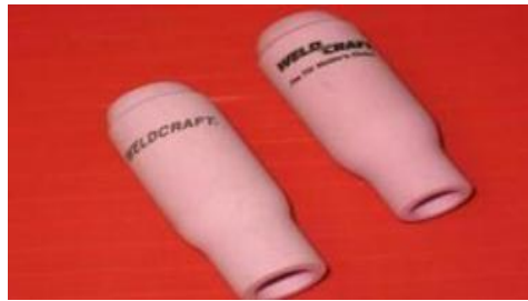
Figure 2.3 - Ceramic cup or nozzle
