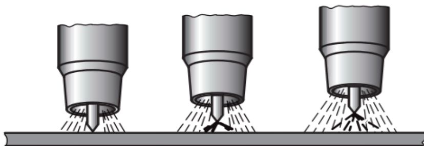
Ignition with the LIFT method.
