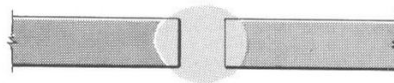
Figure 3.1 The square butt joint is the easiest to prepare and can be welded with or without a filler rod.
