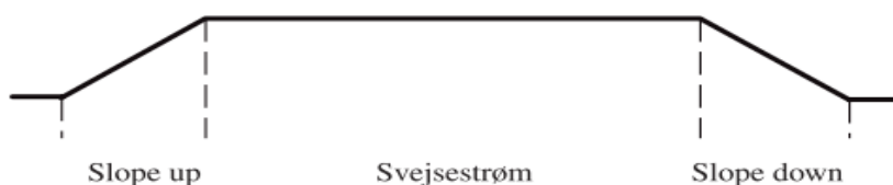
Figure -3.3 Slope facility
