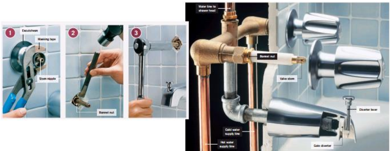
Figure 3.70 Fixing Three-Handle Tub and Shower Faucets
