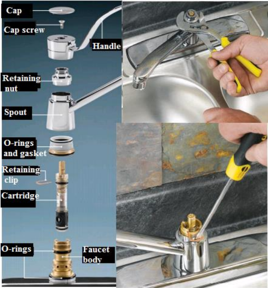
Figure 3.89 One-Handle Cartridge Faucets
