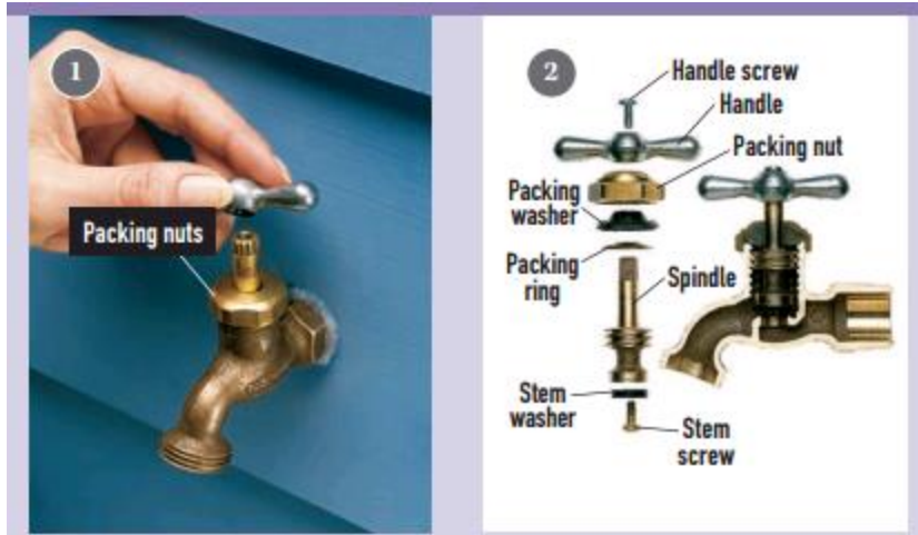
Figure 2.54 Components of hose bib
