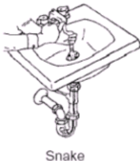
Figure 3.34 Clear up lavatory using snake
