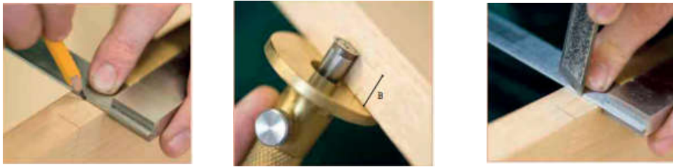
Fig 132 Determine the depth of the dado and mark it
