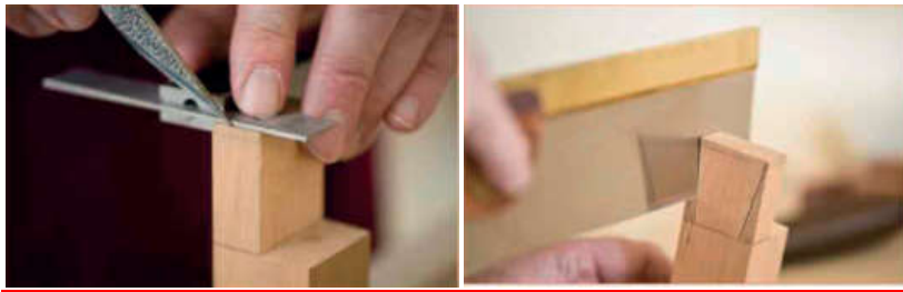
Fig 124 Marking and cutting the side of the tail
