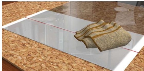
Fig 260 Clean the surface with fine cloth to check the cut
