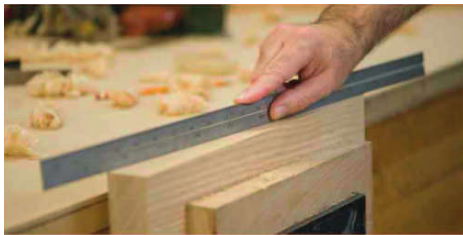
Fig 81 Use a metal ruler to check the end-to-end flatness
