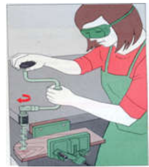
Fig 41 boring a hole
