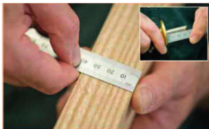
Fig 84 Measure with a ruler and then set the marking gauge to the desired thickness.
