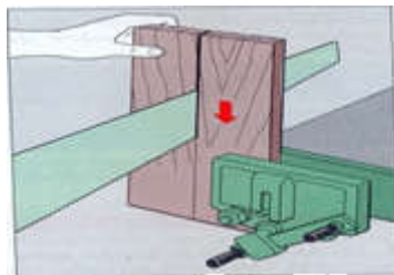
Fig 13 Ripping a board held in vice
