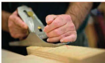
Fig 75 Place the wood in the vise and start the 1 st face side
