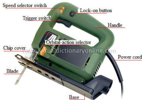
Fig. 58 Portable jigsaws
