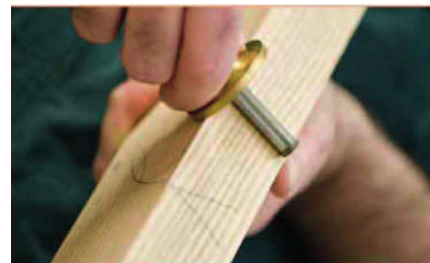
Fig 85 Place the marking gauge against the face side and score the thickness along the edge.
