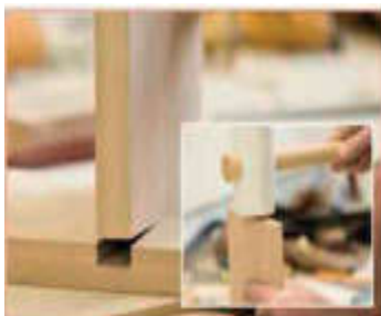
Fig 134 Insert the tenon in the dado Using mallet
