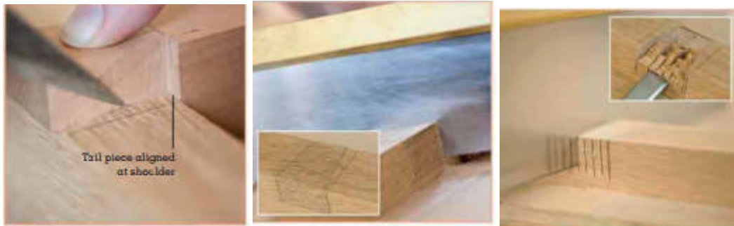
Fig 126 Make relief cuts and chisel it to clean the joint
