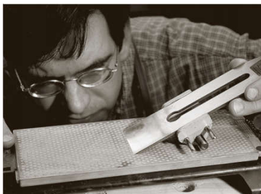
Fig 66 A plane iron clamped in a honing guide
