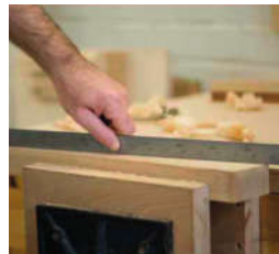
Fig 76 A straight edge such as a metal ruler turned On its edge is used to assess the flatness
