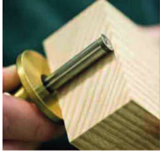
Fig 86 Use the marking gauge to score the thickness along the other edge and both ends of the piece
