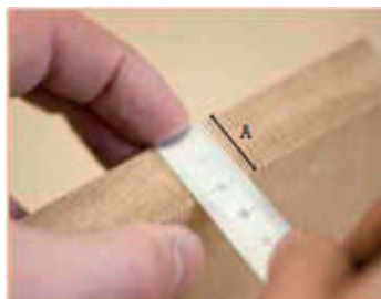
Fig 130 Measure the thickness of the tenon piece
