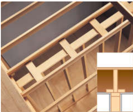
Fig 150 A new wall falls between parallel joists
