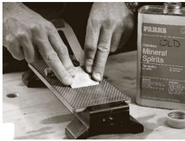
Fig 68 Flat-grinding your cutting bevel
