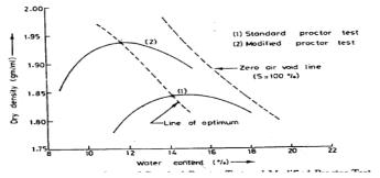
**Fig.** Compaction curves for different compacting effect.
