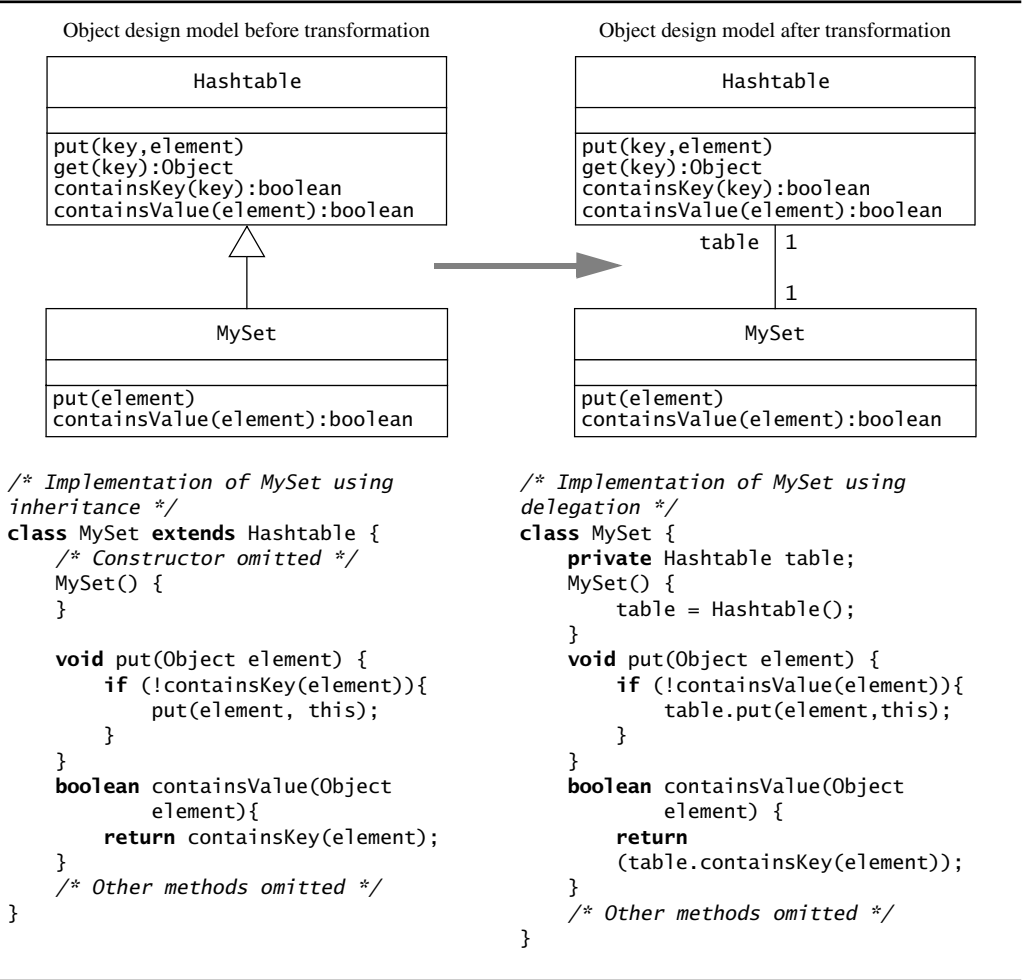
Figure 8-3 An example of implementation inheritance. The left column depicts a questionable implementation of MySet using implementation inheritance. The right column depicts an improved implementation using delegation (UML class diagram and Java).
