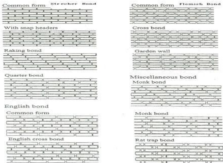
Fig.4. Types of Brick Bond in common use
